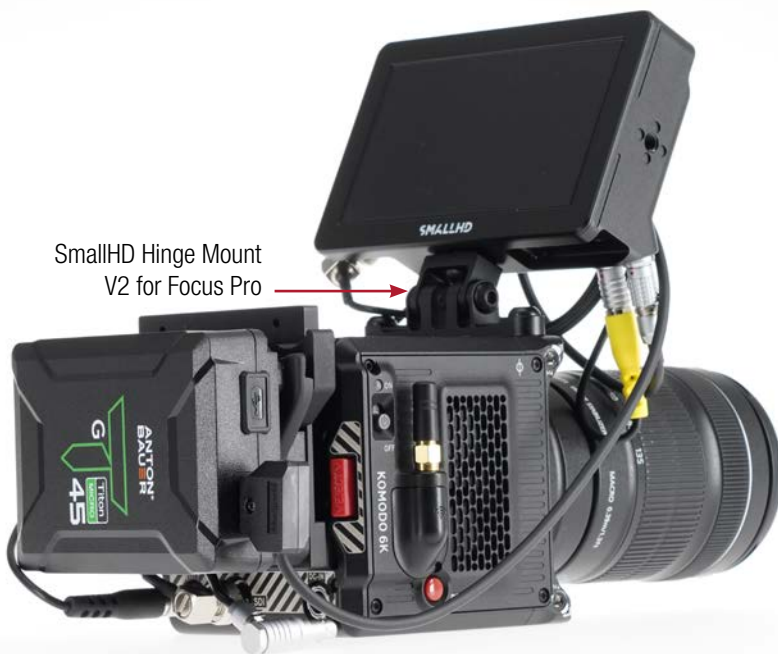
Power from D-Tap to Focus Pro Monitor
