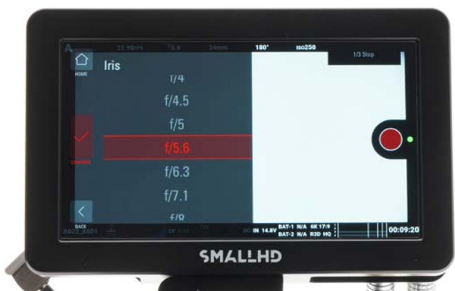
Set lens aperture for enabled lenses.
