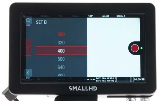
Exposure Index adjustment on touchscreen LCD display.
