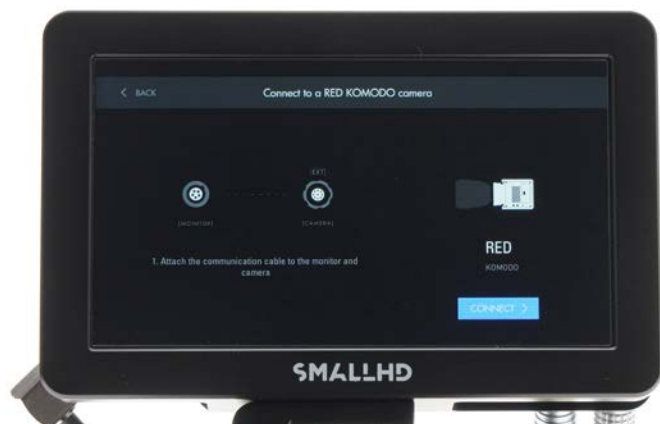
Connect 9-pin KOMODO to 5-pin Monitor control cable.
