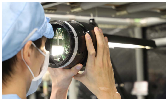
Assembling the optical elements inside the lens barrel.
