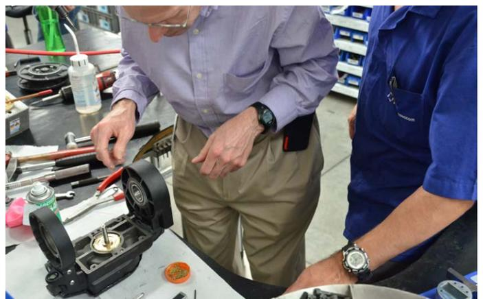
21. Attach shaft and gears connecting crank to lower Whiffletree.
