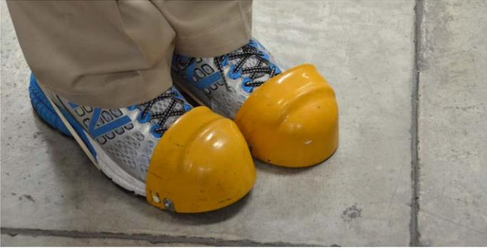
1. Attach toe protectors. Some parts are heavy, like the main casting.
