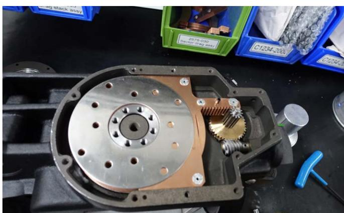
13. Place drag assembly into base casting.
