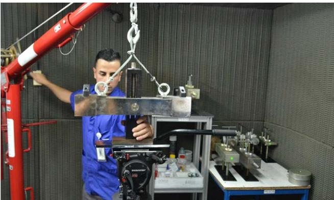
42. He tests the head with various payloads—up to 80 lb.
