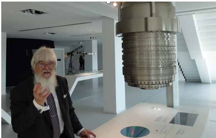
ZEISS Semiconductor Manufacturing Technology (SMT) lens images 20 nanometer structures onto microchips.
