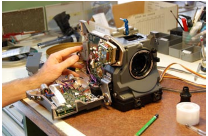
Electronics boards in camera right side cover
