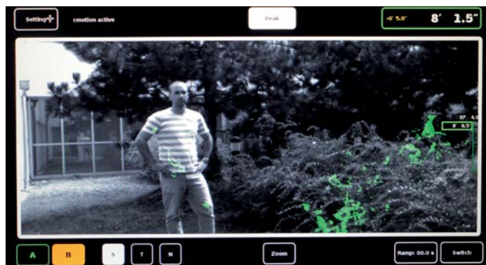
depth of field display — focus set too close, on foreground
