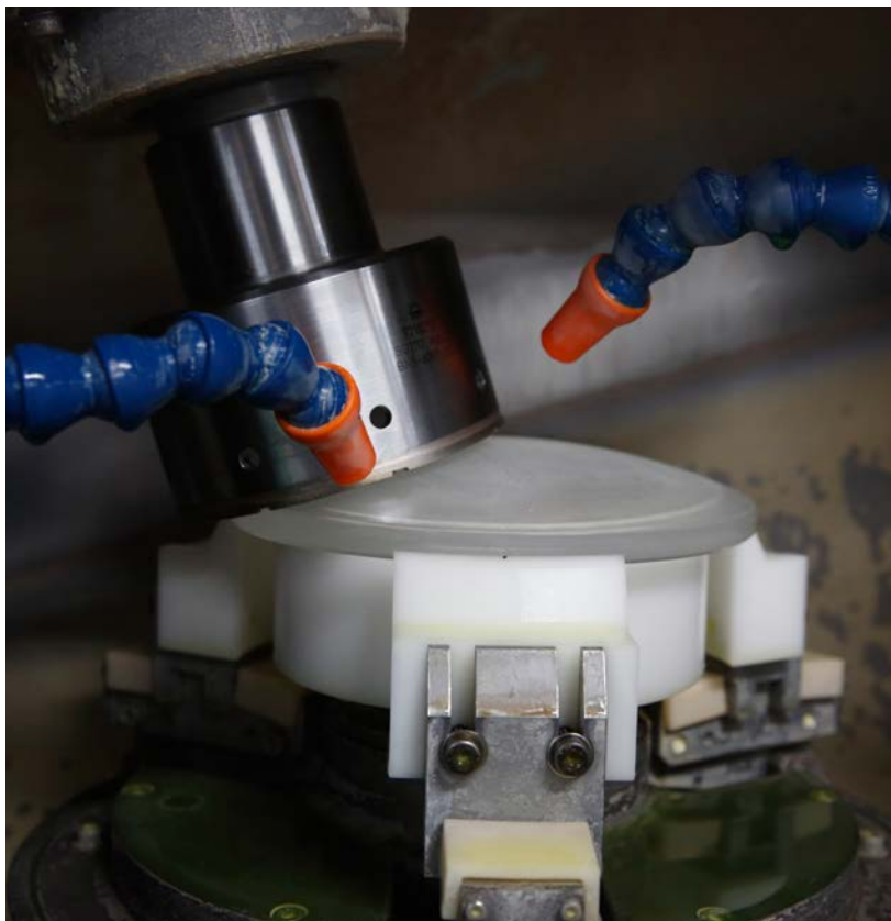
Above: Early in the process—rough grinding an optical element. Below: Lens polishing. Opposite page, bottom: cleaning elements before coating.
