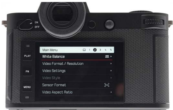
8. WHITE BALANCE is on Menu page 2. Surely we're not wimping out with AWB. Navigate through many choices and pick a numerical color temp.
