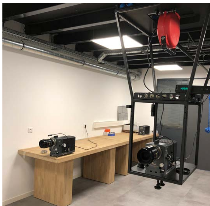
Chrosziel P-TP7 Full Frame projector on Ronford-Baker overhead tracks.
