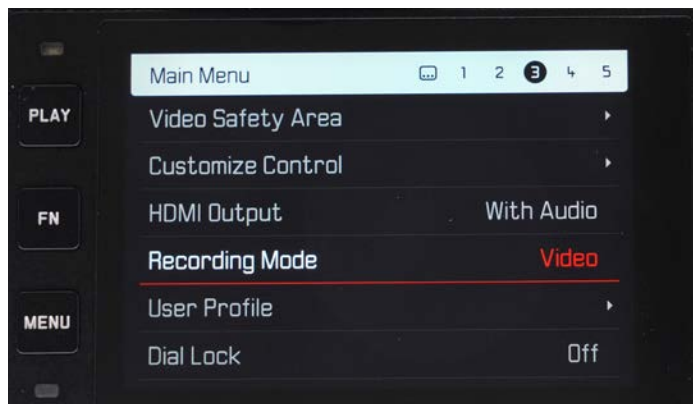
19. As described earlier in frame #5, RECORDING MODE: VIDEO or CINE determines whether you want to see shutter angle or shutter speed, etc.
