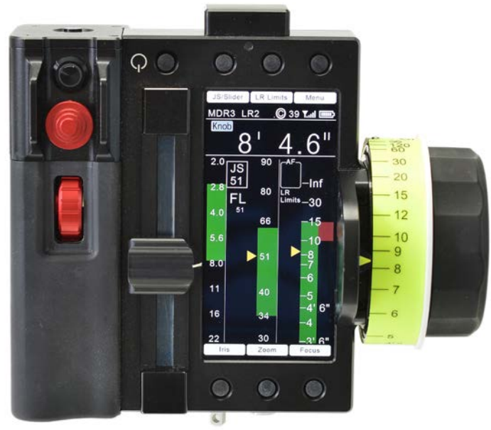
3. Limits are set for Focus, Iris, Zoom, and LR2. The limits for Zoom and Iris are set in the same way as for focus: holding down the respective button while moving the respective control.
