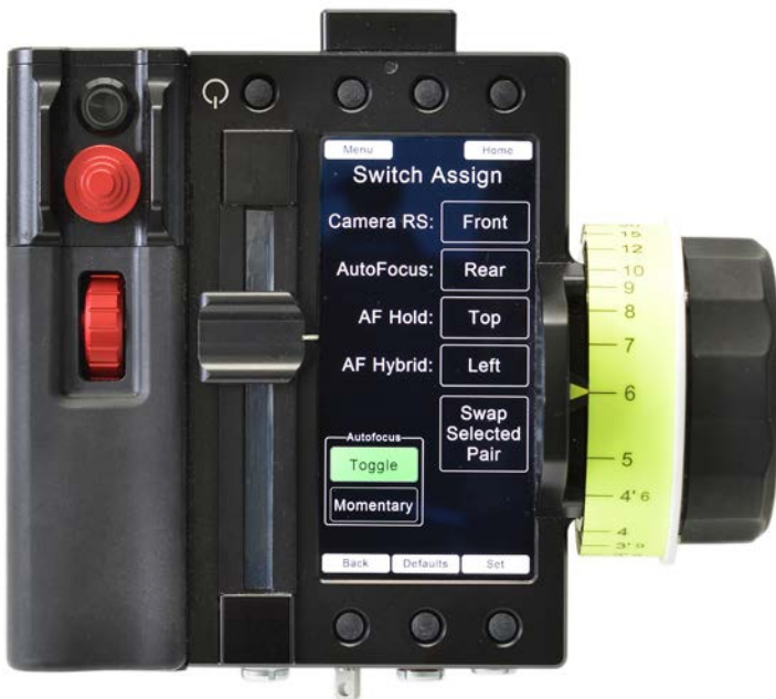
4. Program Switch Assignments. • The Switch functions can be assigned as you like it. • The Autofocus button located on the grip can be programmed to respond only while the button is pressed (momentary) or toggled on/off (toggle).
