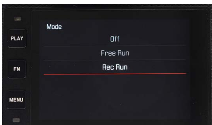
14. RECORD RUN is popular. In FREE RUN, timecode is displayed as time of day whether recording or not. Good for music videos.
