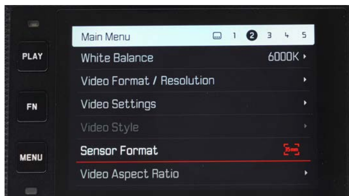
15. SENSOR FORMAT: 35mm. That means Full Format / Entire Sensor. Push joystick to toggle between 35mm and APS-C (cropped image).
