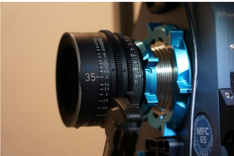
In addition to having a Trioptics MTF Tester, ARRI Rental offices worldwide use the same DENZ MFC 65 lens projector.
