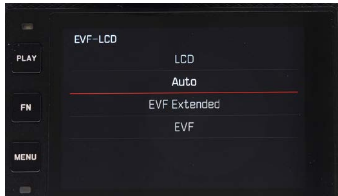
20. DISPLAY SETTINGS adjusts EVF and LCD brightness, EVF frame rate, EVF sensitivity, and whether you want EVF or LCD or both on at all times.
