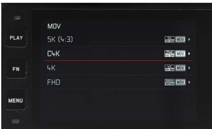
10. Select C4K (4096x2160), jog right to: 24 fps / All-I / 400 Mbps / 4:2:2 / 10-bit / SD & HDMI (Record to internal SD card or externally via HDMI).
