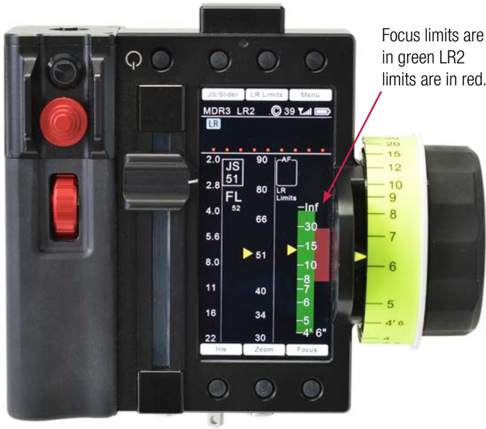
2. This view shows both Light Ranger (LR) and Focus limits set. The display shows dots for the LR2 distance as the subject distance is outside the LR2 distance-limit settings. In Autofocus mode, Light Ranger limits prevent a foreground or background object from causing a focus jump.
