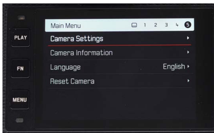
22. CAMERA SETTINGS: change DISTANCE UNITS from Metric to Imperial, turn camera beeps on or off, and to enable USB battery charging. So, that should have been about 45 seconds. As always, menus change as firmware is updated, and there are other ways to do these tasks.
