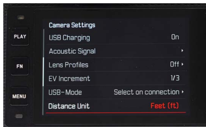
22. CAMERA SETTINGS: change DISTANCE UNITS from Metric to Imperial, turn camera beeps on or off, and to enable USB battery charging. So, that should have been about 45 seconds. As always, menus change as firmware is updated, and there are other ways to do these tasks.
