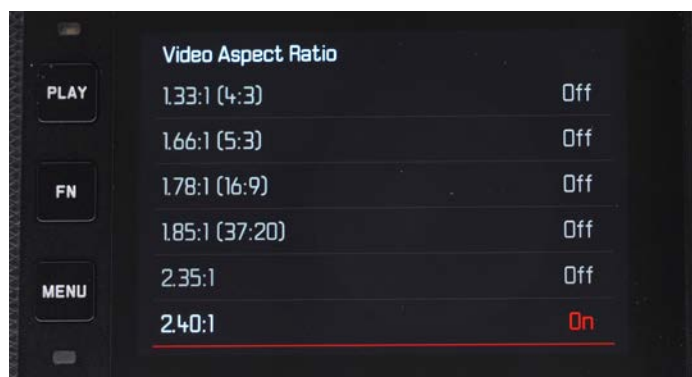
16. VIDEO ASPECT RATIO: push joystick to select one or more framelines. This does not crop or window the recorded image.
