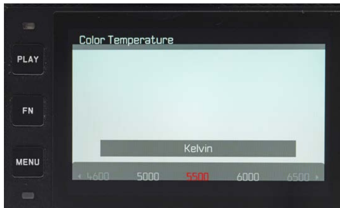
8. WHITE BALANCE is on Menu page 2. Surely we're not wimping out with AWB. Navigate through many choices and pick a numerical color temp.
