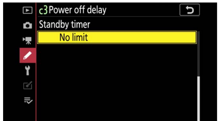
6. CUSTOM SETTING MENU > C TIMERS / AE LOCK > C3 POWER OFF DELAY > STANDBY TIMER > NO LIMIT...so camera does not go into power saving standby in the middle of a take.
