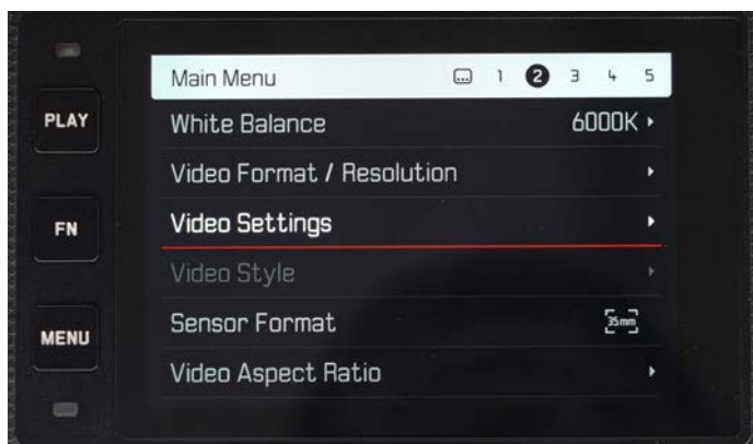
11. VIDEO SETTINGS: Video Gamma L-Log (Leica Log). From L-Log, you can jog right and adjust sharpness. Instead of L-Log, you can choose HLG.
