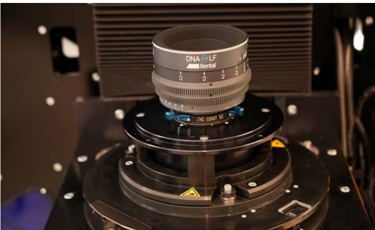
Christian Agerer “driving” the custom-designed Trioptics MTF optical testing device. As mentioned, each ARRI Rental facility in Munich, Berlin, London, Burbank and New York has commissioned one of these. ARRI Cine Technik also uses this machine in manufacturing and QC of Signature Primes. In this photo taken with an ARRI DNA LF 35mm at T2, note how the extremely tuned field curvature blurs and distorts the keyboard, above at right.
