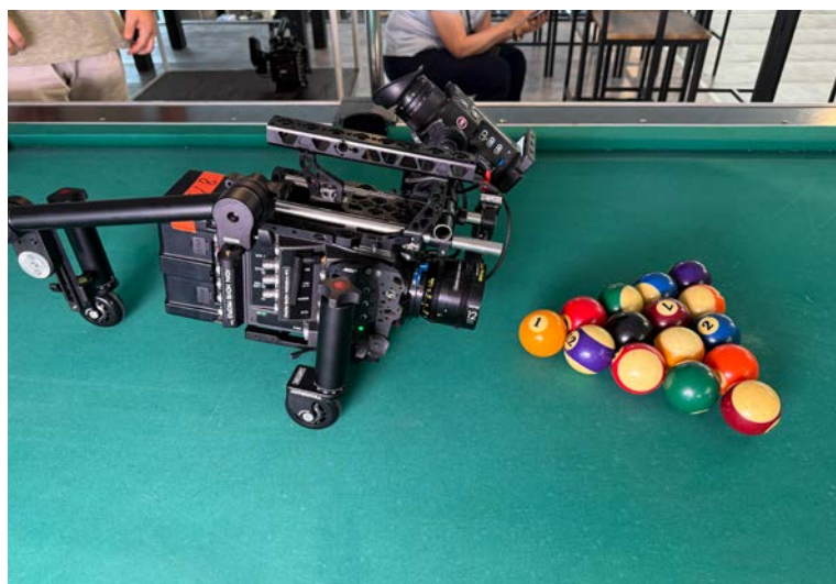
HyperRoll with ALEXA 265 and DZOFILM Vespider 12mm T2.8 lens.
