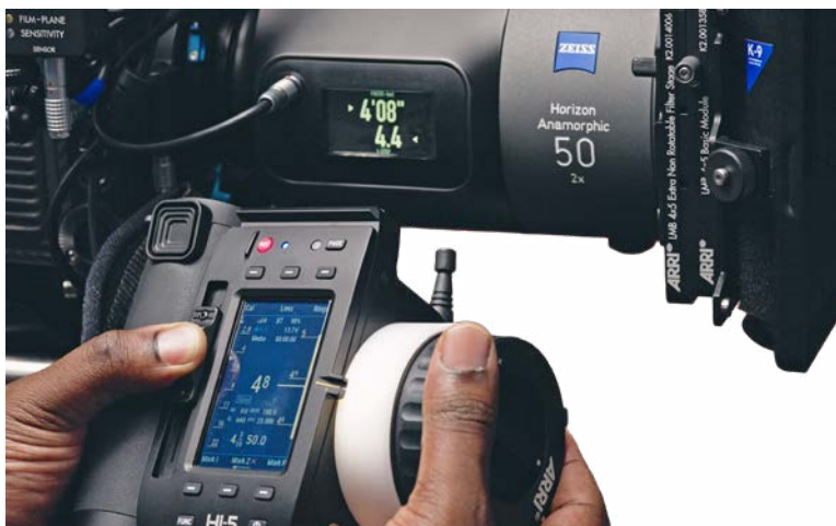
ARRI Hi-5 controlling Horizon lens via LCUBE LBUS-to-Serial converter.
