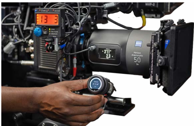
Horizon Anamorphic controlled by ARRI OCU-1 (Operator Control Unit).
