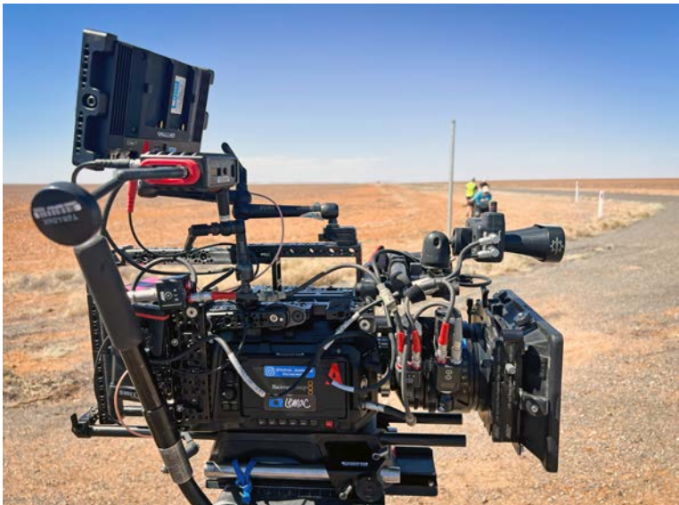
A Camera build: URSA Cine 17K 65 with T-Tuned Blackwing7, Cine RT Focus-Bug, ARRI ECS, Teradek and SmallHD high-bright monitor.
