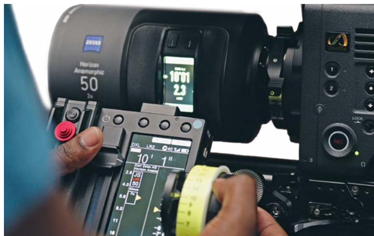
Preston HU-4 controlling Horizon lens via MDR connected to 7-pin Lemo.
