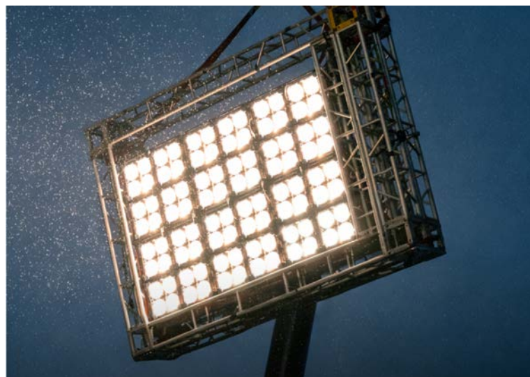
6x Four-Fixture-Frames with Fresnel Lenses = 24x Matrix 2500 units. 24 x 2500W=60,000W (60K). Like a "96-Light NANFAY."
