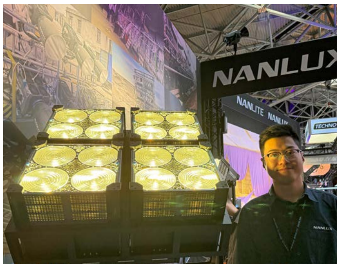
Andy Lin with four prototype Matrix 2500C fixtures in a Four-Fixture-Frame. 4 x 4="16-Light". 4 x 2500W=10,000W (10K).
