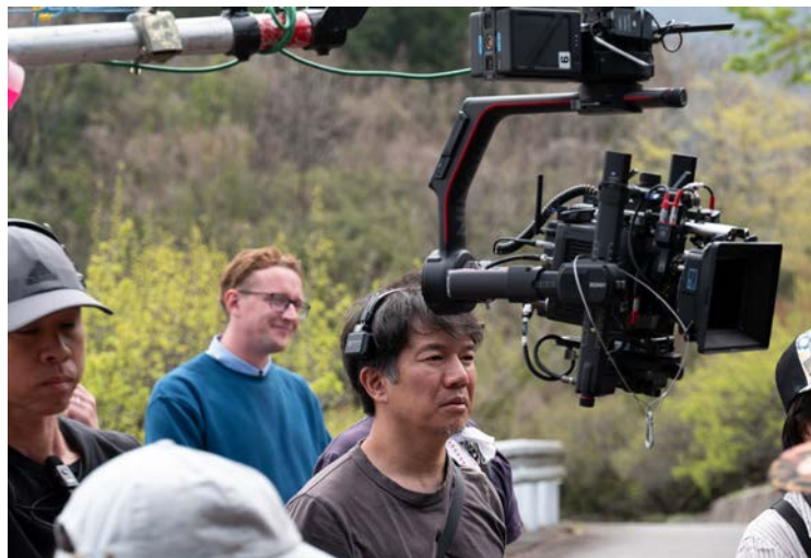
ALEXA Mini LF on speedrail crane with DJI Ronin 2. Photo: Searchlight Pictures/James Lisle.
