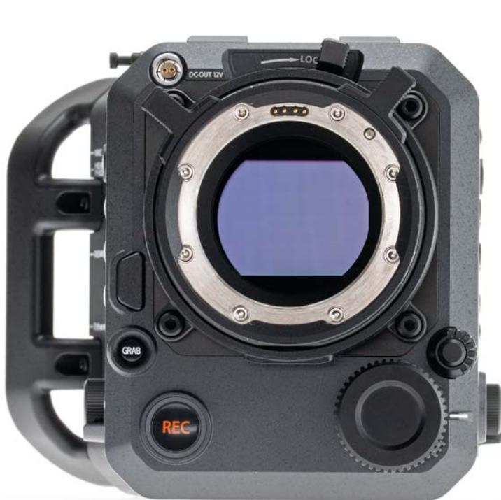
PL Mount Adapter by Fujifilm comes with the GFX ETERNA 55 camera.
