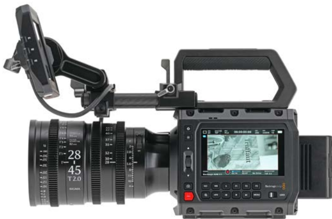
PYXIS Monitor mounted in front for shoulder-resting or handheld.
