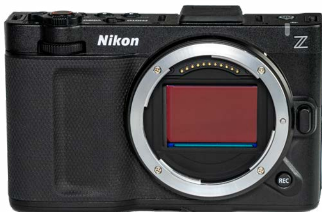
24.5 Megapixel Full Frame Partially Stacked CMOS Sensor
