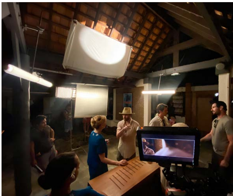
Litemat 2L source pushing through a 4x4 diffusion. Astera Titan tubes with white noodles cut to size for extra diffusion.
