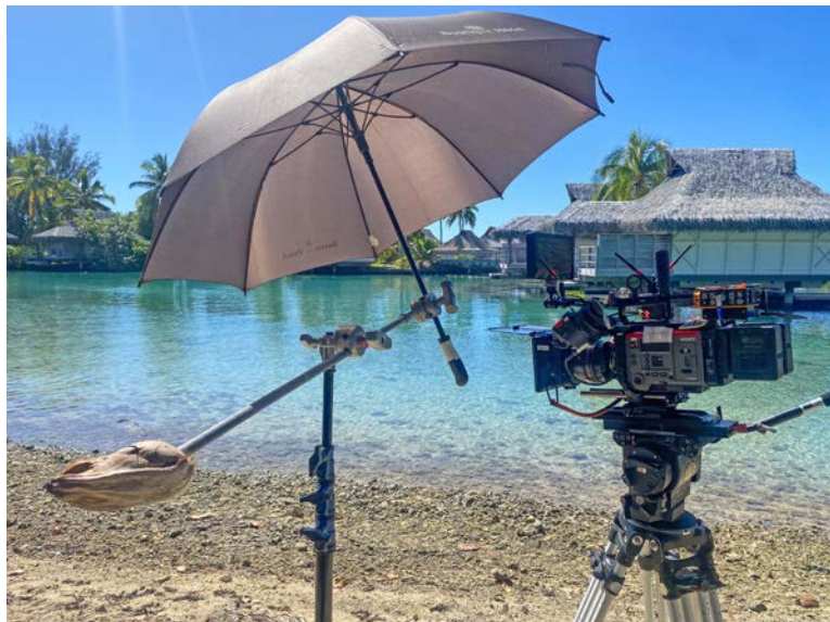
Coconut safety bumper for C-stand gobo arm.
