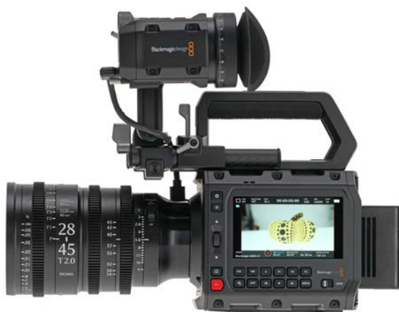
EVF bracket arm positioned vertically.
