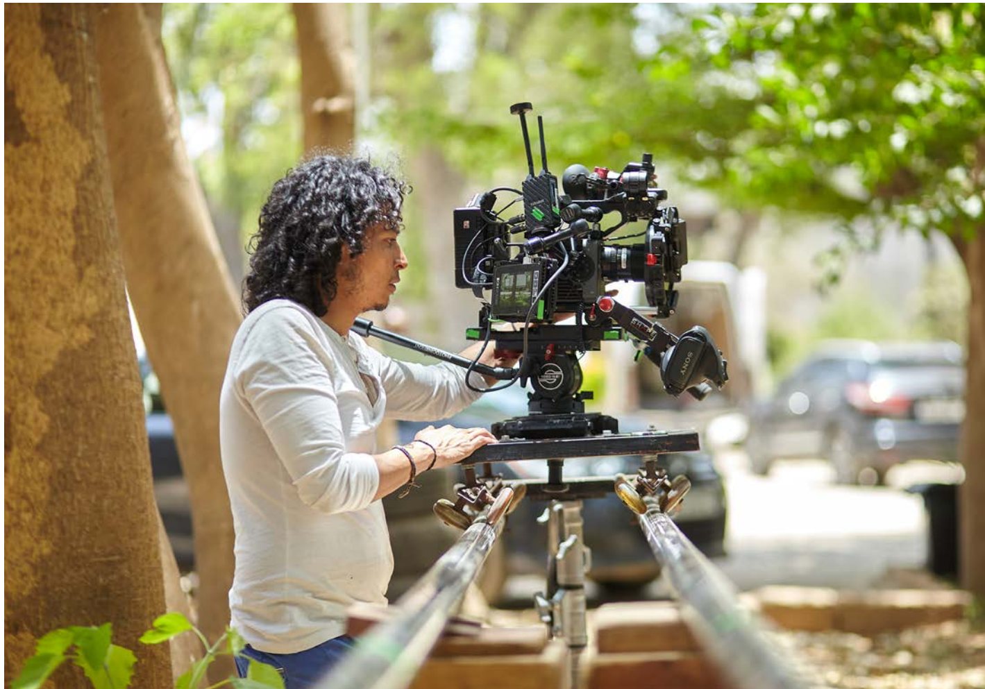
FX9 on a slider with Sachtler Video 15 head, Cooke SP3, SHAPE WLB right handgrip extender, SmallHD monitor, Teradek Bolt.
