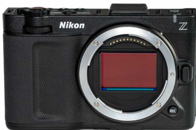
24.5 Megapixel Full Frame Partially Stacked CMOS Sensor
