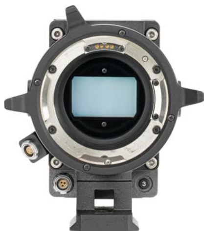
Sony PL Mount attaches over E-mount with four 3mm hex screws
