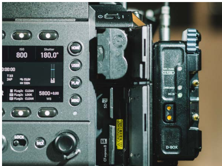
Internal battery and media bay, with a Wooden Camera D-Box and Anton/Bauer battery plate in back.
