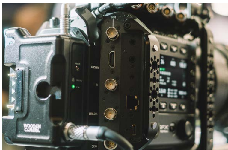
SDI, HDMI, TC, Genlock, DC In, Mic, Headphone, Remote, Ethernet, USB-C.
