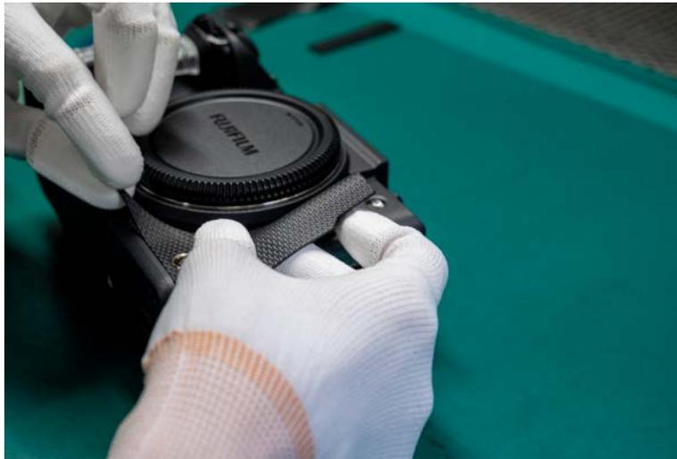
Ms. Oizumi attaches a textured, non-slip surface to the camera body. It takes her less than 3 minutes from start to finish. At least two months are necessary to become proficient at this.
