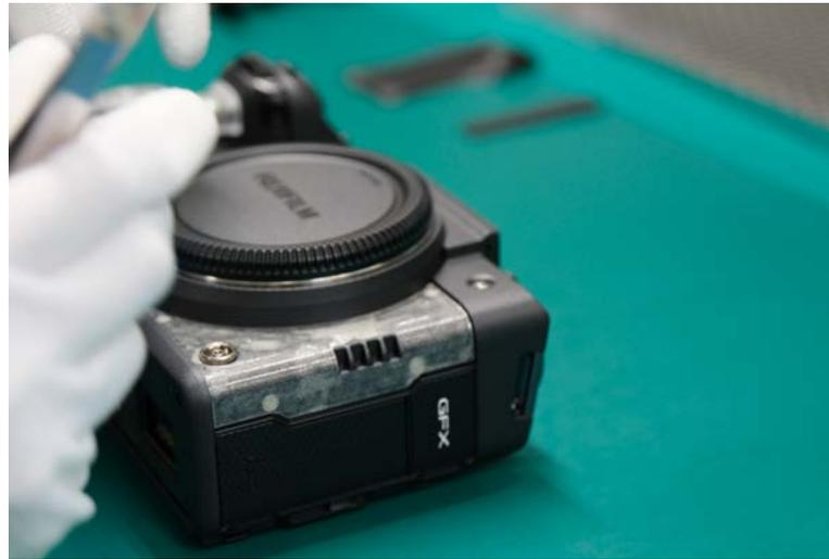
At 1/80th sec and f/4.0, Ms. Oizumi's fingers are a blur as she smooths the double-sided super-sticky surface to the camera body. For example, even one grain of sand (62 microns) would be annoying to the touch. Imagine how a bump, bubble or ridge would feel?
