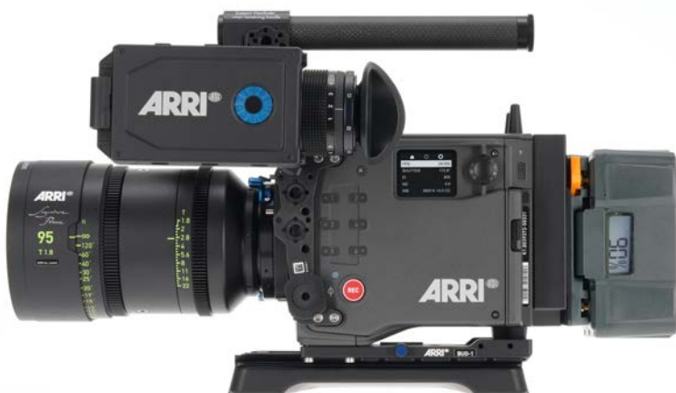
When shoulder-resting, do not assume this is like an Arriflex 235. The curved base is there for cooling. Use a shoulder pad that allows air to enter the camera from the bottom.
