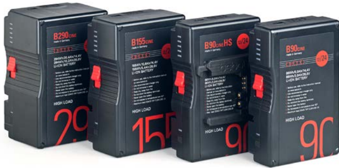
Bebob 14.4 / 28.8 Dual-Voltage B-Mount Batteries. There are currently four different Bebob B-Mount batteries available now – from the B90cine with 86Wh capacity to the B155cine (156Wh) and the B290cine (285Wh). Bebob, based in Munich, developed the B-Mount system three years ago. It has a new, multi-voltage-capable interface that has been shared as an open, manufacturer-independent industry standard.
