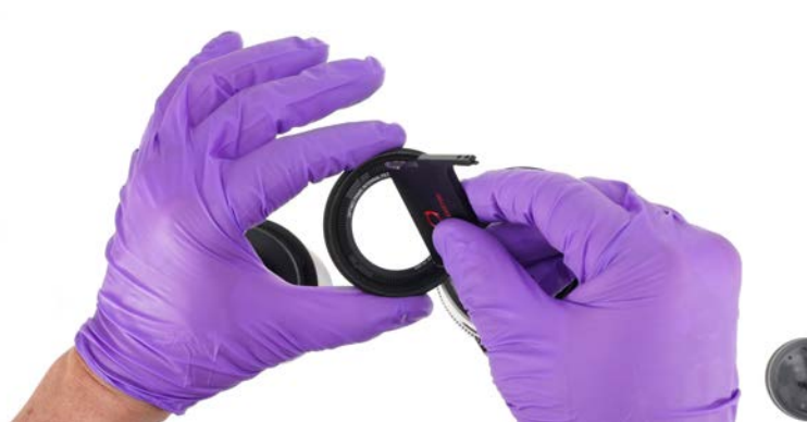
14. Remove the retaining ring with the internal elements spanner.
