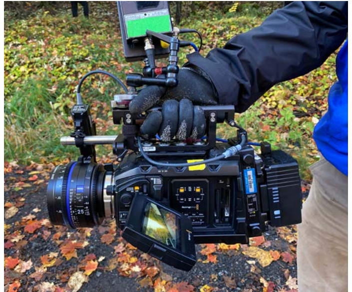
ARRI SXU wireless iris control unit powered with Wooden Camera D-Box.
