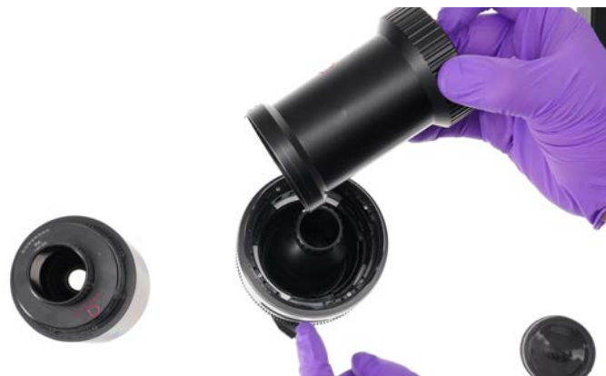
10. Remove the IOP Outer IOP Tool.
