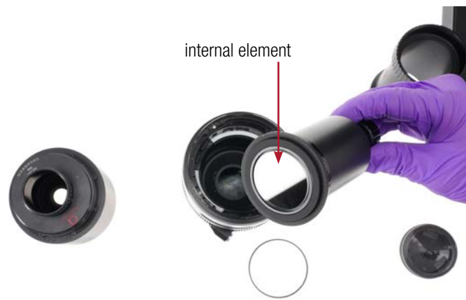
12. The iris assembly is seen below the internal element. This is where you begin to swap the iris assembly using the same inner IOP tool to remove it.
