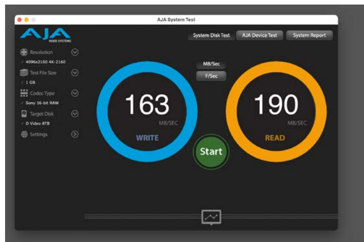
AJA System Test reading an 8 TB spinning hard drive. Note: 163 MB/sec (megabytes per second = 1304 Mbps (Megabits per second)) 190 MB/sec (megabytes per second = 1520 Mbps (Megabits per second))
