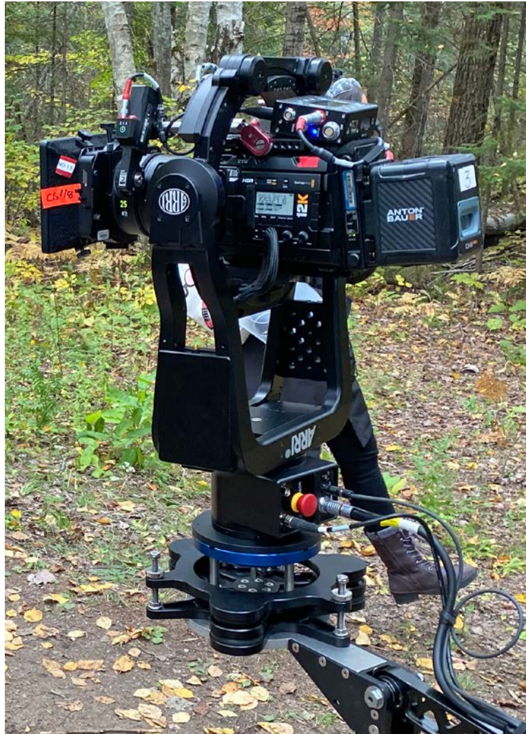
ARRI SRH-3 remote head with vibration isolating Flowcine Black Arm on Zero FXS Electric Motorcycle.
