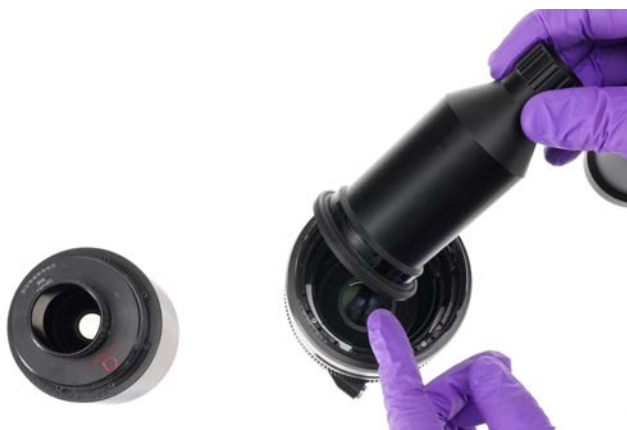
11. Extract the Inner IOP Tool with the internal element and retaining ring attached.
