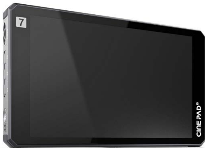
CINEPADS 7 front and left side: Menu dial and 3 user buttons.
