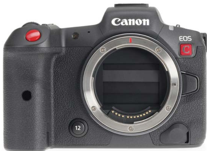
Shutter closes when camera is off—helpful when changing lenses.
