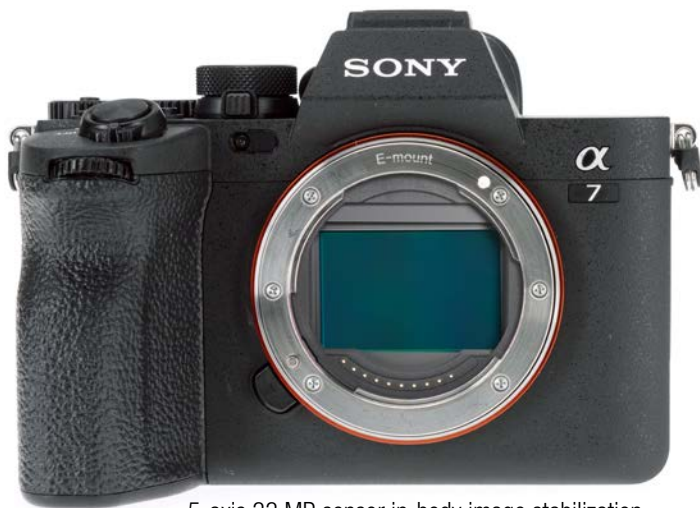
5-axis 33 MP sensor in-body image stabilization
