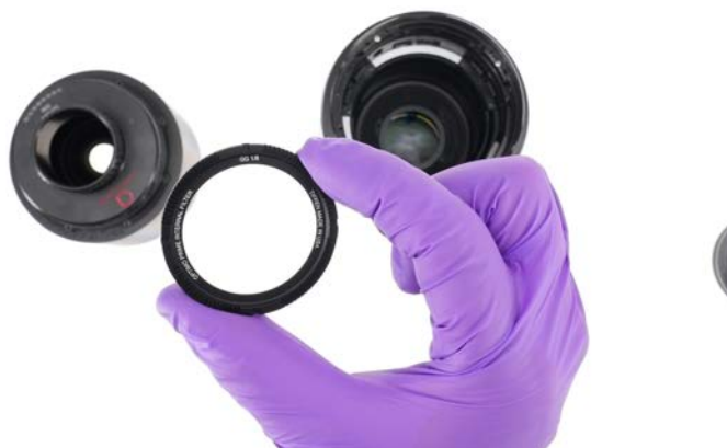
15. Out comes the internal element, ready to be swapped for another.
