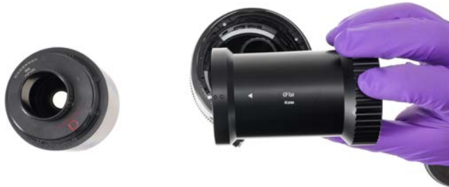
9. Insert the Outer IOP Tool to unscrew the IOP retaining ring.
