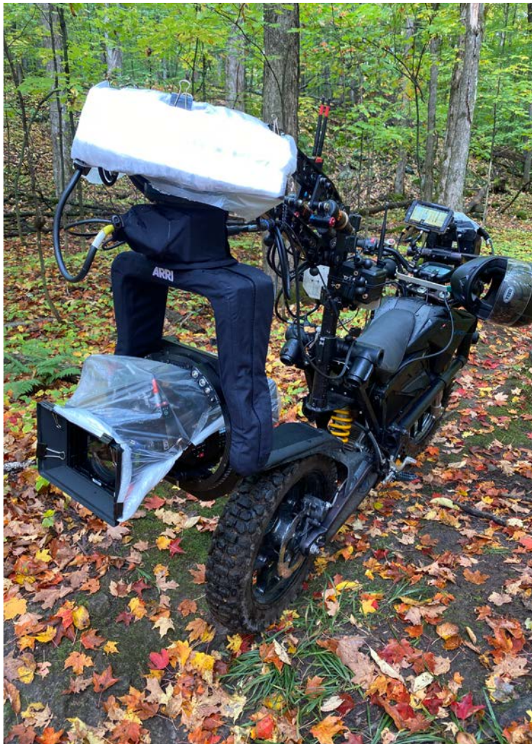
ARRI SRH-3 remote head with vibration isolating Flowcine Black Arm on Zero FXS Electric Motorcycle.
