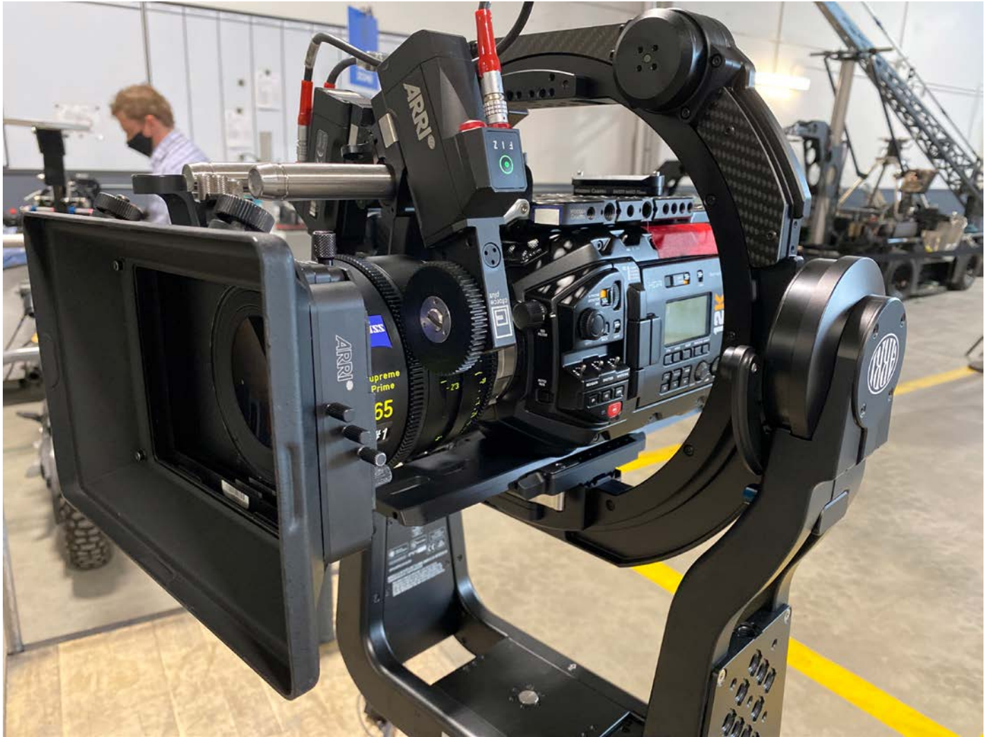
URSA Mini Pro 12K with ZEISS Supreme Prime on ARRI SRH-3 Remote Head.
