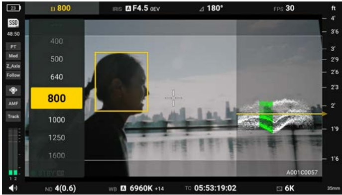
1. Most camera settings are available at the touch of the touchscreen or the push of a button. Adjust with a finger swipe or by turning the monitor dial. The EI button selects from 200 - 12,800.
