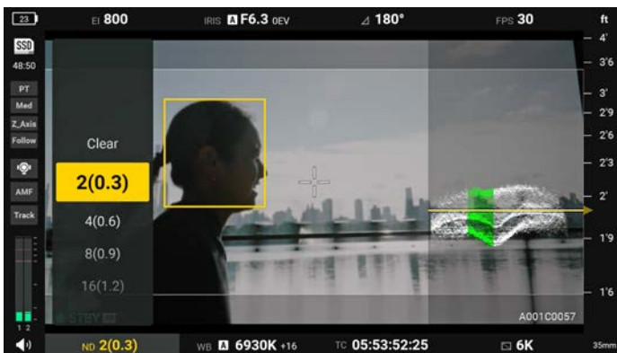
7. Select internal NDs of Clear and ND.3 (1 stop) to ND2.7 (9 stops).
