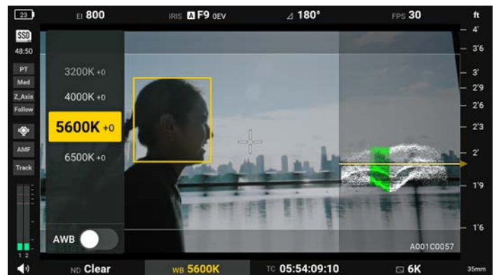
8. Press and hold White Balance to measure WB or add custom settings.
