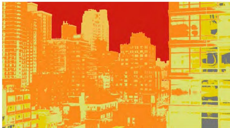
Over exposed. The sky is +4. Only a few windows are 18% gray. From FDTimes office with VariCam LT feeding an AJA U-Tap SDI to Quicktime screengrab.
