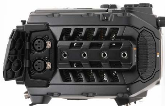
Top: 2 XLR 3-pin audio connectors are located under rubber flap at rear. The 4 mounting threads are 1/4-20.
