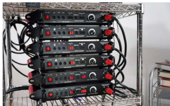
6 Bi-Color dimmable DMG Lumiere fixtures are controlled by 6 SL1 drivers with 24' cables. I decided to stack them. Sort of a DMX alternative, but it is quick and easy.
