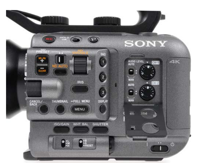
Detail of Audio Controls with Door Open.
