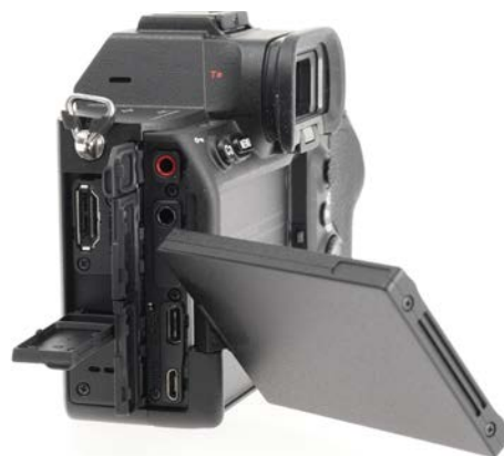
Touchscreen monitor flips out and rotates to the side.
