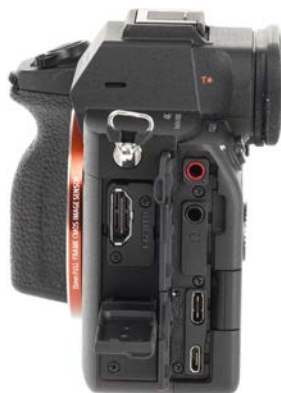
Connections: Full size HDMI Type-A and USB-C that also charges battery.
