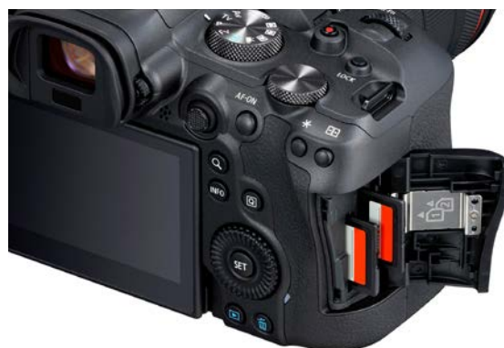
The R6 has two SD UHS-II card slots.
