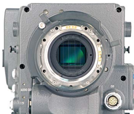
Left: Blue Streak Effect filaments in ARRI ALEXA.
