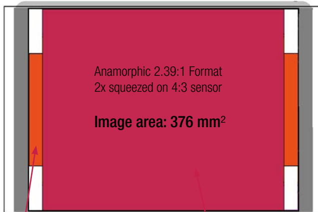
Fig 2. Anamorphic 2.39:1 on 4:3 ALEXA Sensor
