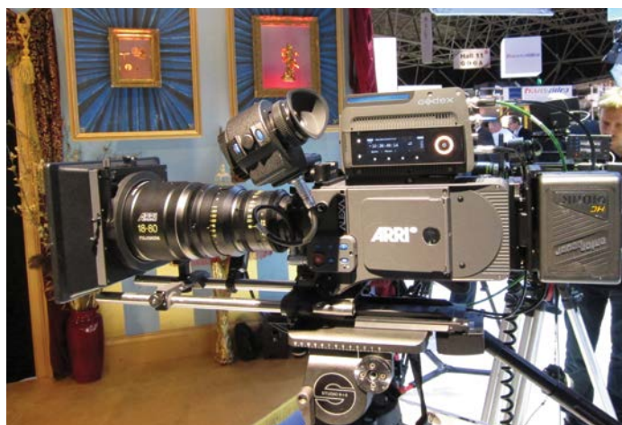
ALEXA Plus with Codex Onboard Digital Recorder, ARRI/Fujinon Alura 18-80 mm zoom, Anton/Bauer onboard battery.
