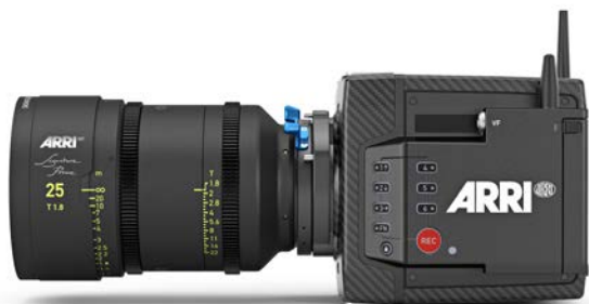
The bare essentials. Camera left. 6 User buttons. REC button. VF connector
