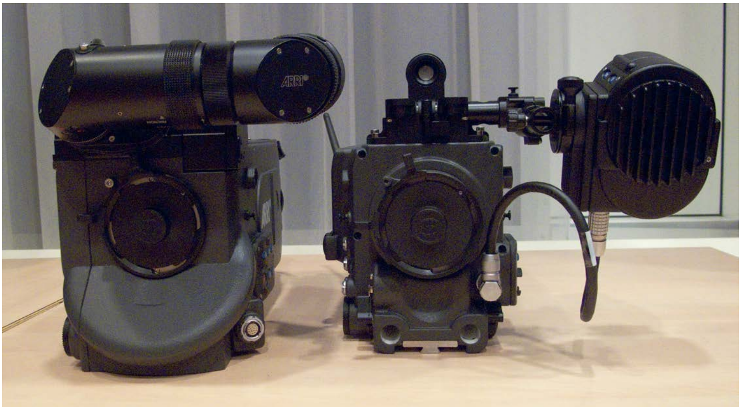
Above: front view of Alexa EV pre-prototype with electronic finder, and lightweight 15mm supports under PL mount.
