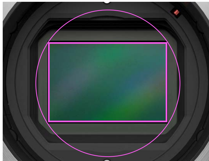
ALEXA LF Open Gate 4480 x 3096: 44.71 mm image circle 36.70 x 25.54 mm image area
