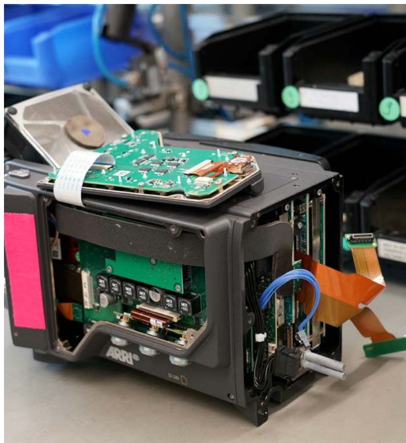
Printed Circuit Boards and fan go inside the rear camera body housing.
