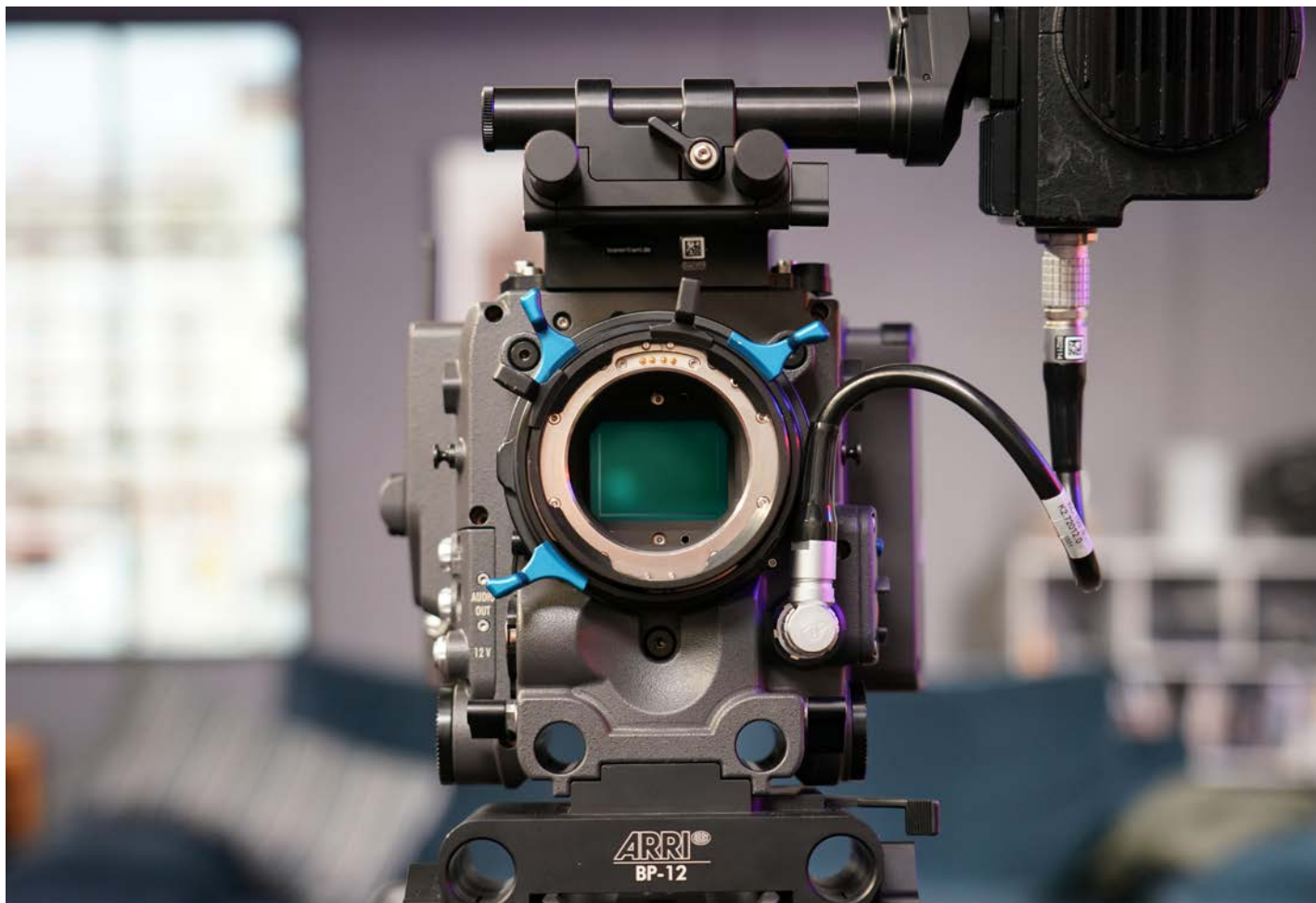
PL-to-LPL adapter accepts any PL mount lens on ALEXA LF. The PL mount has 2 traditional black ears. The LPL mount has 3 blue ears.
