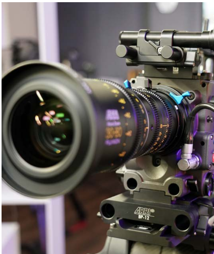
PL-to-LPL adapter accepts any PL mount lens on ALEXA LF. The PL mount has 2 traditional black ears. The LPL mount has 3 blue ears.
