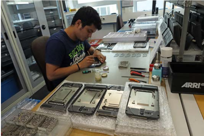
Preparing SXT camera left side media drive doors
