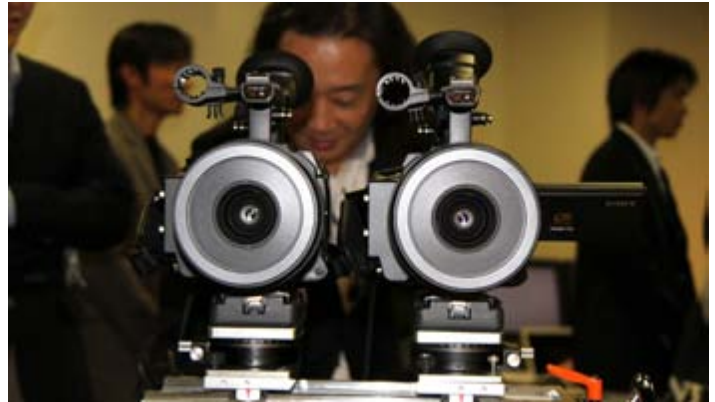
Above: Two F3 cameras set up on a 3D side-by-side rig.
