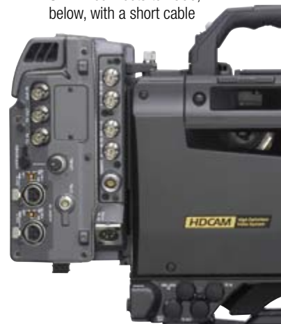
SR-R1 connects to F900, below, with a short cable
