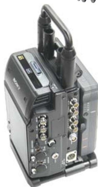
SR-R1 connects to F900 with a short cable
