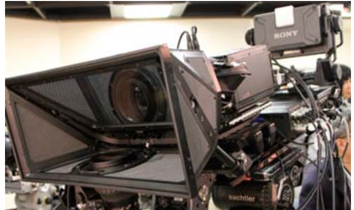
Below: Two P1 box cameras on an Element Technica Pulsar mirror rig.
