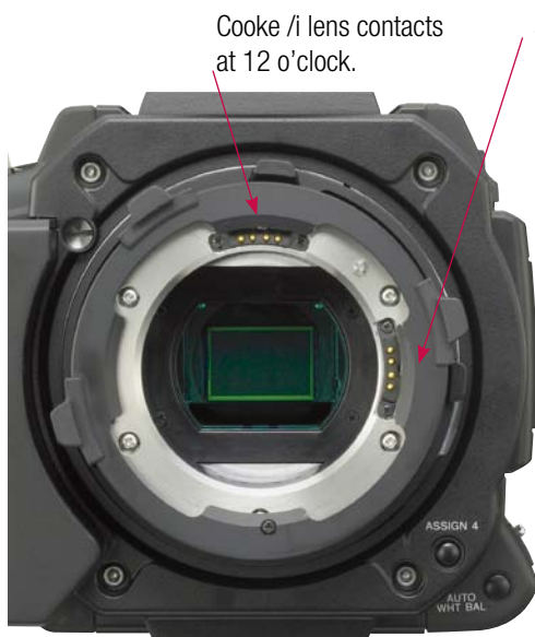
ZEISS/ARRI LDS lenses have contacts normally positioned at 3 o'clock.
