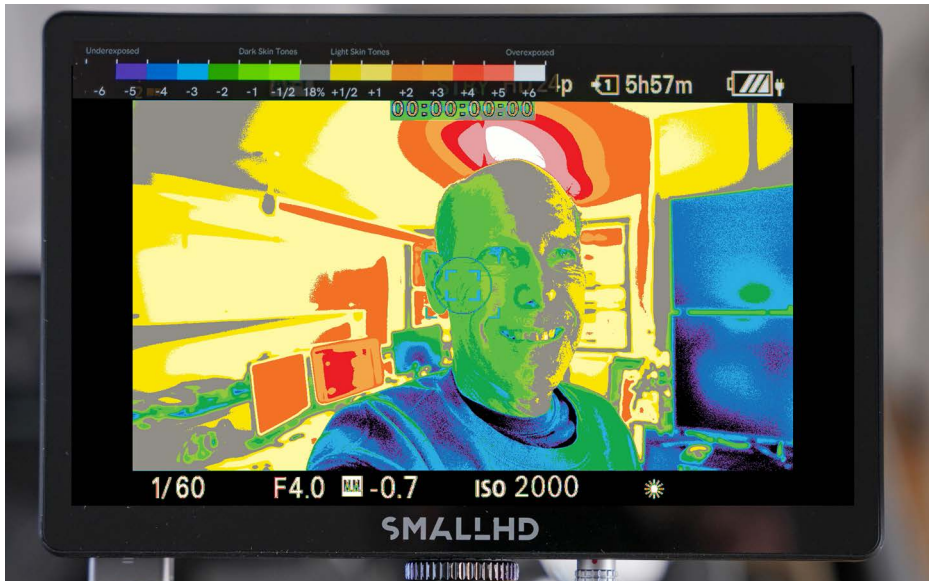
SmallHD Cine 7 with EL Zone active. Exposure is set for camera right side of face (18% gray).
