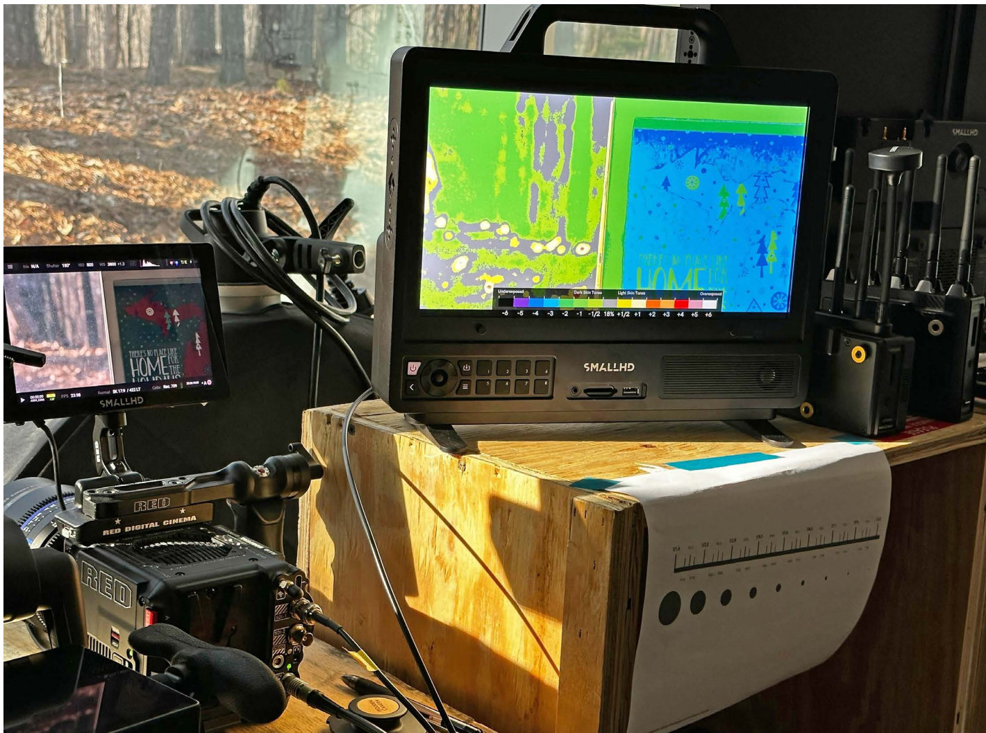
Above: EL Zone being tested at SmallHD in Cary, NC. RED V-RAPTOR's SDI output is connected to a SmallHD Cine 13 with EL Zone enabled.
