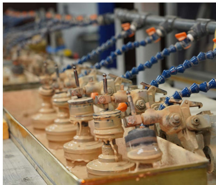
The polishing compound is an abrasive slurry of Cerium Oxide.
