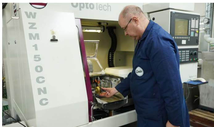
Of course, many lenses undergo high-speed CNC edging.
