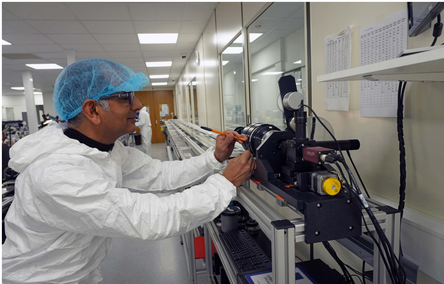
Raj Mistry hand calibrates the focus scale of each lens. After this, the focus barrel is laser engraved.
