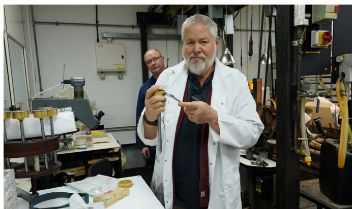
Separate the element from the spindle by gently tapping shaft. Les Zellan demonstrates.
