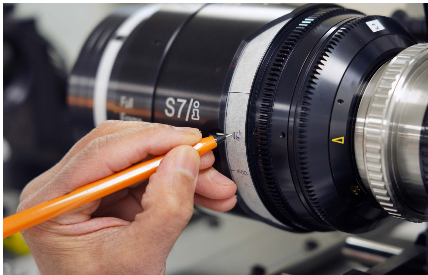
Raj Mistry hand calibrates the focus scale of each lens. After this, the focus barrel is laser engraved.
