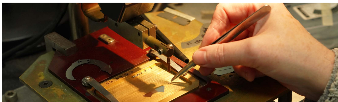
Iris leaf pins are welded into position.
