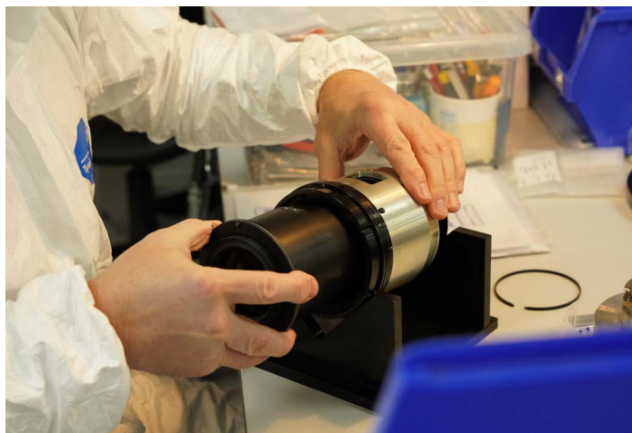
Inners (sub assemblies) slide into outers.
