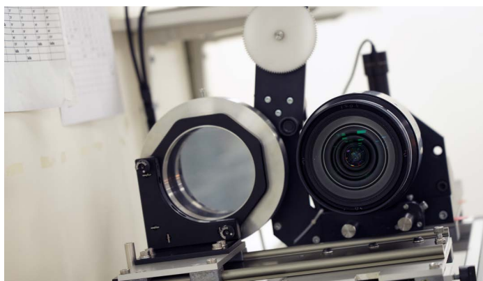
Infinity is established with a supplemental mirror.
