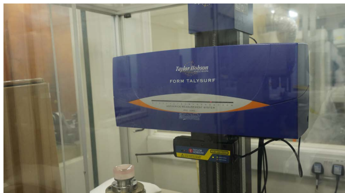
The Form Talsurf measures aspheric polishing inconsistencies. The original Talsurf 1 by Taylor & Hobson Talsurf was introduced in 1941 to accurately measure surface texture.
