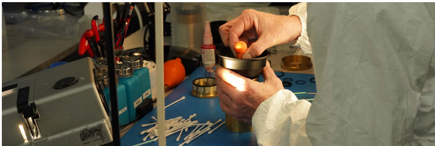
Above: the precise edging done earlier pays off as lenses mount inside barrels. Below: Inside a flow booth, the cams mate with cam followers.
