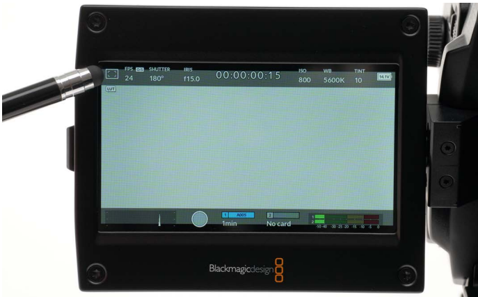
1. Touch the top left framing icon to set frame lines.
