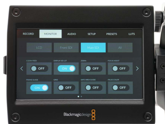
6. Main SDI is the BNC output at camera rear, usually going to Video Village.
