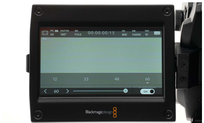
6. Choose FPS on top line. Select off-speed rate at bottom. Turn ON or OFF.
