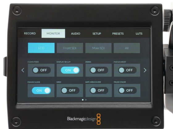
4. Monitor Settings Page. LCD is the swing-out monitor display.
