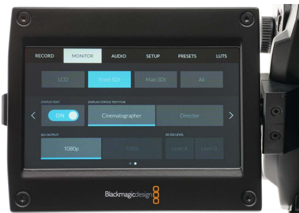
5. Front SDI is usually the camera operator's EVF.
