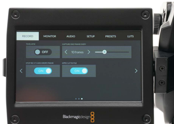
3. APPLY LUT IN FILE and STOP RECORDING IF CARD DROPS FRAME.
