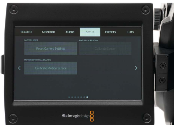
9. When all else fails, Reset camera to factory defaults.
