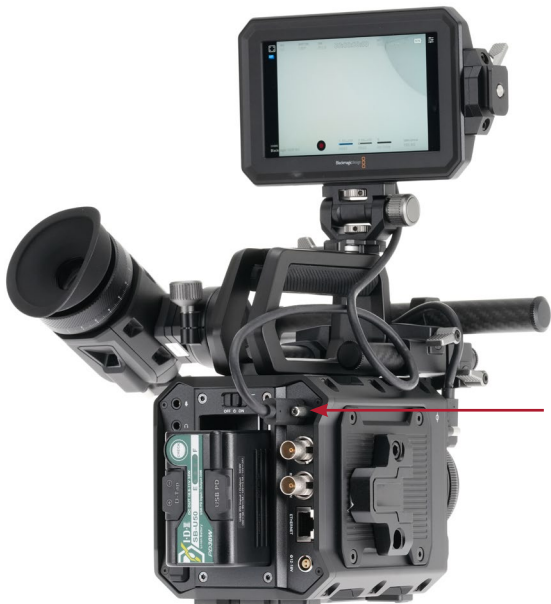
PYXIS Monitor connected to the rear USB-C port via a single USB-C DisplayPort / Power cable.
