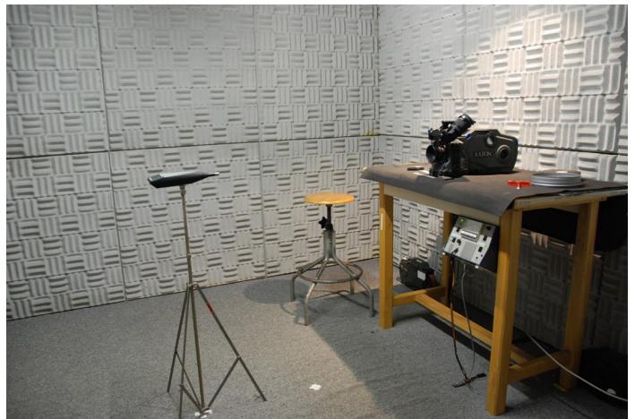
Penelope is tested in the sound isolation room. The cameras are better than 23 db.
