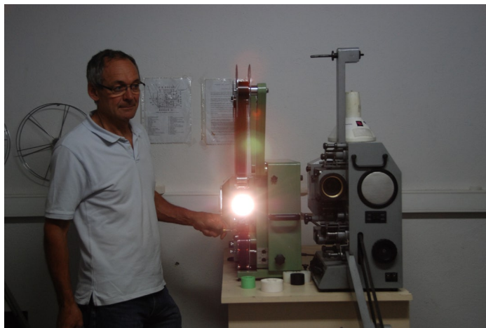
Every camera is tested for steadiness. Alain Guerre-Dailly projects a film test.
