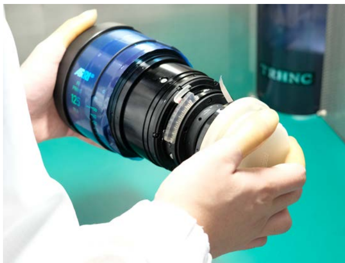
Calibrating LDS-2 lens metadata on prototypes.
