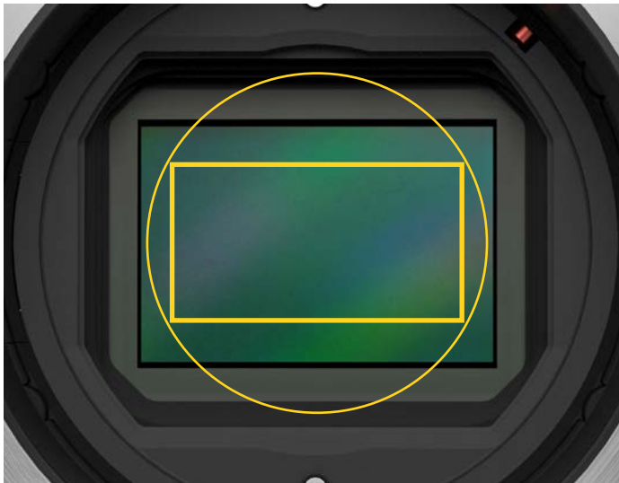
ALEXA LF 16:9 sensor mode 3840 x 2160 (4K UHD) 36.35 mm image circle, 31.68 x 17.82 mm image area
