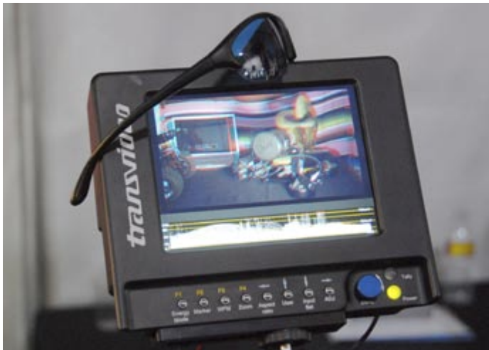
Monitors include Waveform, Vectorscope, Histogram and Overexposure Control.
