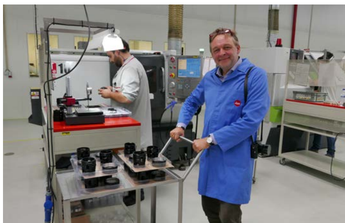
Gerhard Baier and a cart of Summicron-C mechanical assemblies
