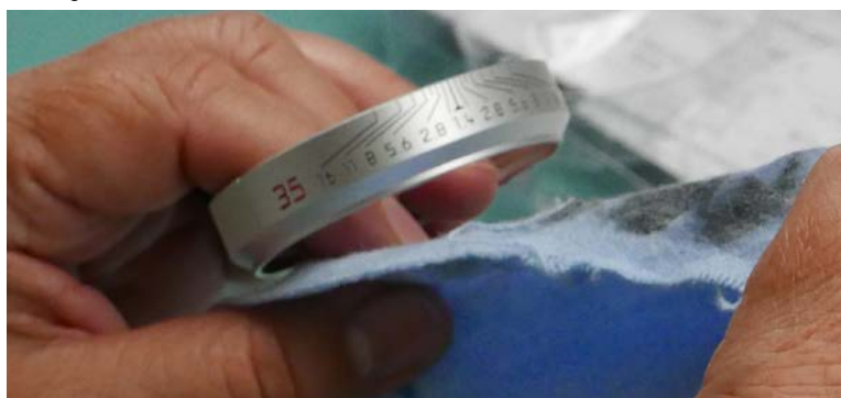
The engraved numbers and letters are filled with paint and then the excess is wiped clean, leaving color only in the recessed areas.
