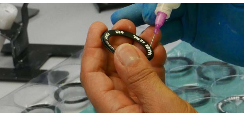
The engraved numbers and letters are filled with paint and then the excess is wiped clean, leaving color only in the recessed areas.
