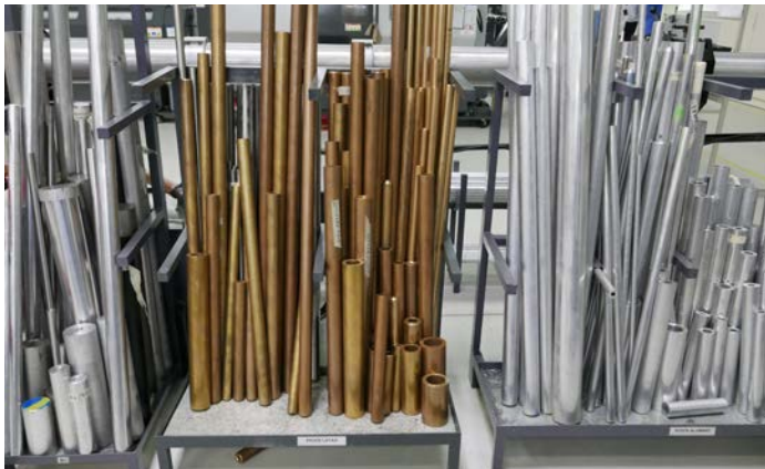
Lens barrels and mechanical sub-assemblies begin life as solid blocks or tubes of aluminum and brass, steel, magnesium and titanium.
