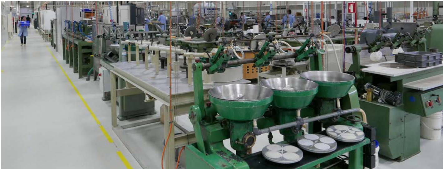
Blocks of glass take shape in the early stages of polishing in a huge machine room, above. Traditional method, below left. Computerized, right.
