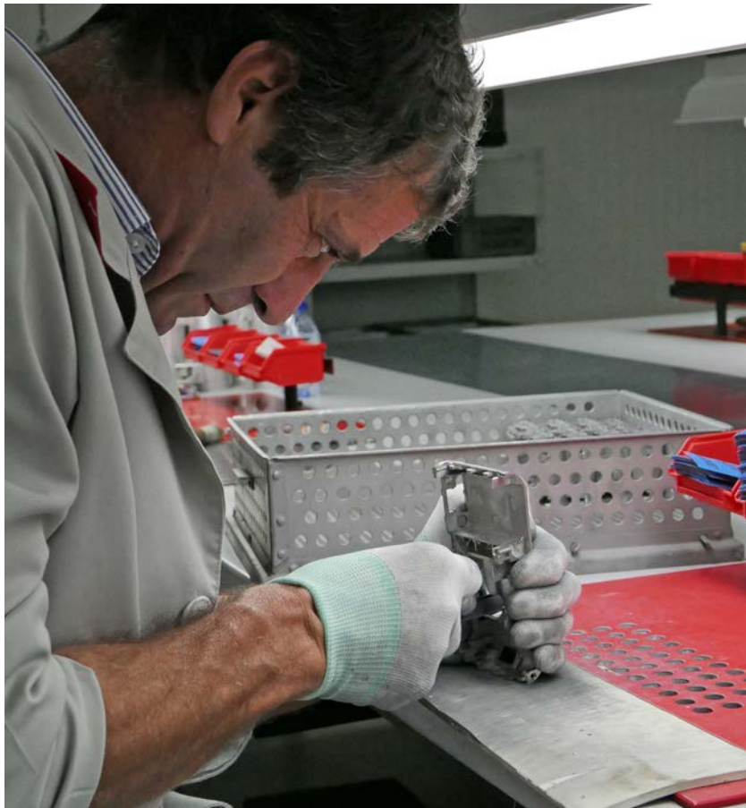
Leica M cameras are finished by hand—with meticulous attention to detail, polishing and smoothing edges.
