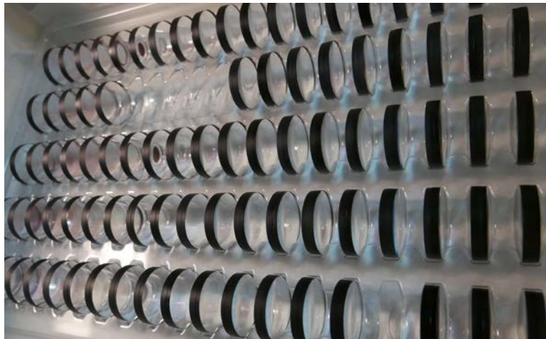
Edges are treated with a special matte black paint to further reduce reflections—and then loaded into trays in preparation for assembly.
