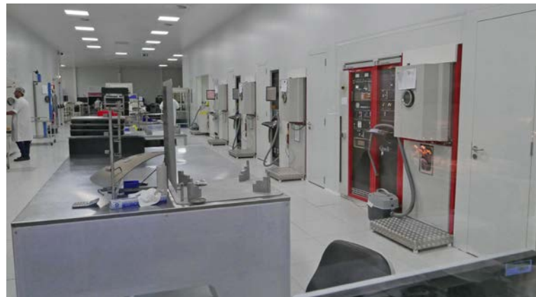
Machines vaporize and deposit the metals onto the glass elements.
