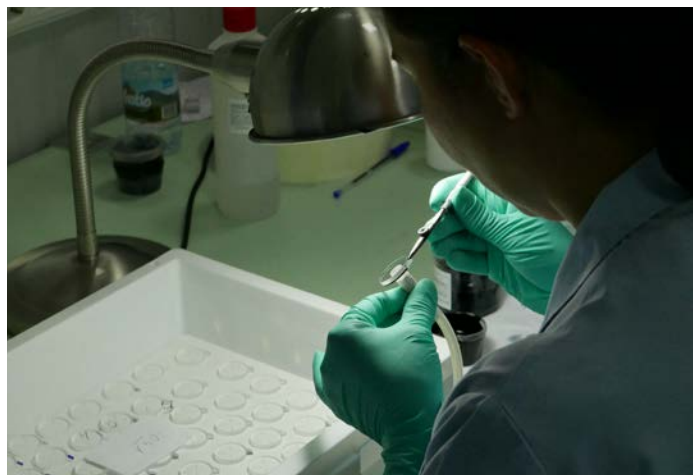
Edges are treated with a special matte black paint to further reduce reflections—and then loaded into trays in preparation for assembly.
