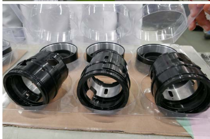
The lens barrels are anodized in-house.
