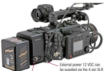
be supplied via the 4-pin XLR connector on the camera.
