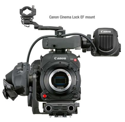
Canon C700 comes with the choice of two mounts. The Cinema Lock EF is a more rugged mount than the ones found on still cameras. This one has a locking ring and supports bigger, heavier lenses. FFD=44 mm. ID=54 mm.
