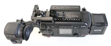
4. Top Handle attaches with 2 screws. OLED EVF-V70 comes with an adjustable support and cold shoe mount. (Note: the Anton Bauer Cine 150 battery shown here is V-Mount.
