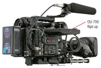
9. OU-700 Remote Operation Unit attaches to the camera right side and mimics all the functions of the built-in Main Display. It conveniently flips up for access to the CFast and SD card slots.
