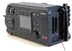
2. A multi-pin connector is revealed. The Codex Recorder connects here. CDX-36150 records 4K RAW uncompressed up to 120 fps.
