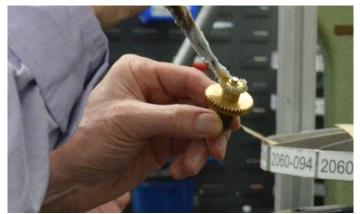
4. Apply grease to O-ring of pan drag adjustment control.
