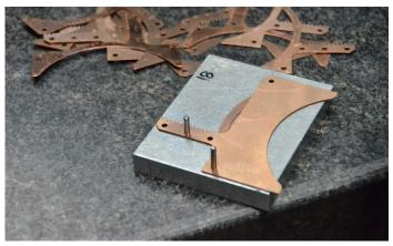
9. Stack one set of copper plates together with spacers on a jig.
