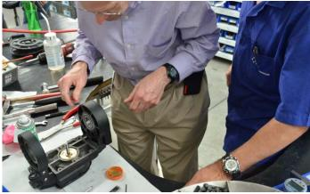
21. Attach shaft and gears connecting crank to lower Whiffletree.
