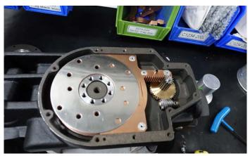
13. Place drag assembly into base casting.
