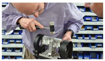
23. Installing lower Whiffletree, crank pin and block into counterbalance housing. Yikes, I have managed to get it jammed!
