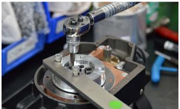
14. Secure and tighten with torque wrench.
