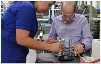
20. Upper Whiffletree shafts on top part of head's tilt assembly.
