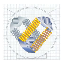
OConnor's **dual axis counterbalance system** involves two sets of springs attached to the Upper-Wiffletree on top. A Wiffletree evens out unequal forces. The name comes from the yoke that connects two horses pulling a carriage. The higher the number of the crank, the more the springs extend, and the more weight they can support.
