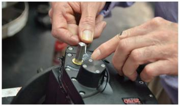
34. Place pan and tilt drag readout disks.
