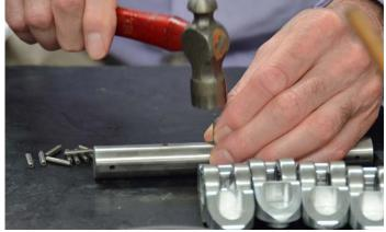
19. Line yokes up on shaft and secure with pins
