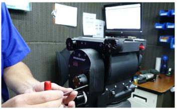
39. QC is done on every head. Each screw, bolt and setting is checked. The inspection of every head takes 1.5 hours.
