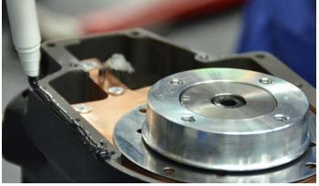
16. Prepare base with airtight seal. It will be filled with fluid later on.
