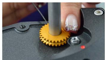
31. Gears for balance indicator attached.
