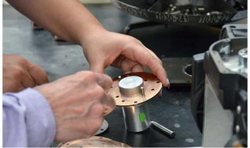
10. Stack the other set of plates on the shaft.
