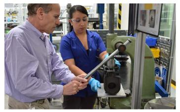
3. Press bearing assembly onto main shaft of casting
