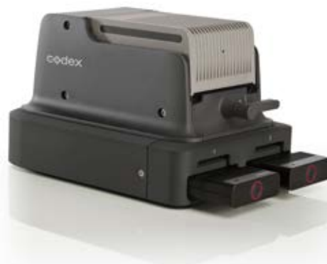
If you don't have a Vault (but you should), the Transfer Station M for Mac OS X will wrangle your data from Codex Datapack on top to Codex Transfer drives on bottom, and to connected hard drives as well.
