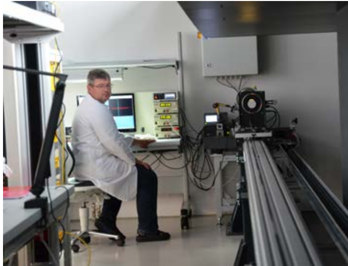
Now it gets really interesting: a very high-tech focus-scale indexing system on a 60' long "railroad" moves an MTF target to each marked distance to be engraved on the focus barrel.
