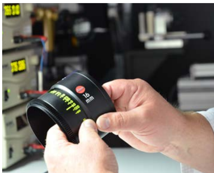
Assembly begins: the mechanical focus components are prepared prior to installing the optical elements
