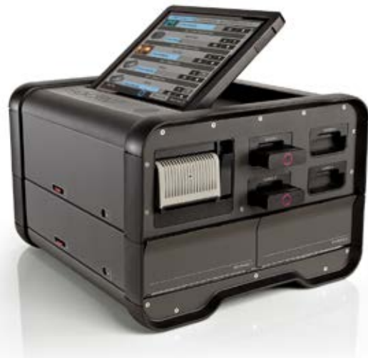
Codex Vault with two storage bays added for internal hard drives.
