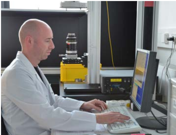
Measuring air gaps of completed lens
