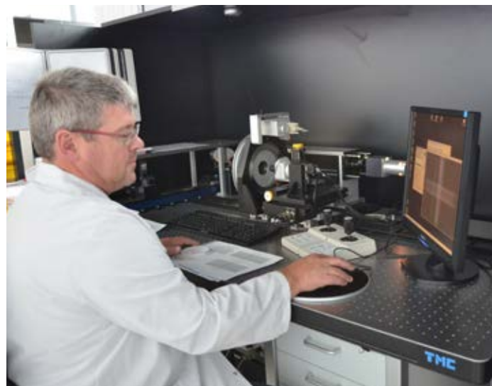
Racking lens focus remotely while looking at a computer read-out of MTF contrast. When the optimum setting is achieved, he clicks "save," and the setting is stored. The data goes to a laser engraving machine. Each focus ring is therefore optimized for each lens.
