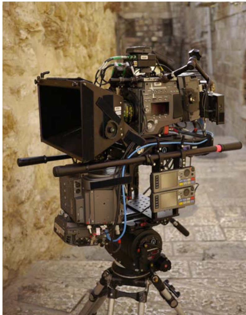
Below: Two F65 cameras on CC3D Rig in Alleyway in Muslim Quarter of Jerusalem's Old City. Photo: Francis Hanneman.
