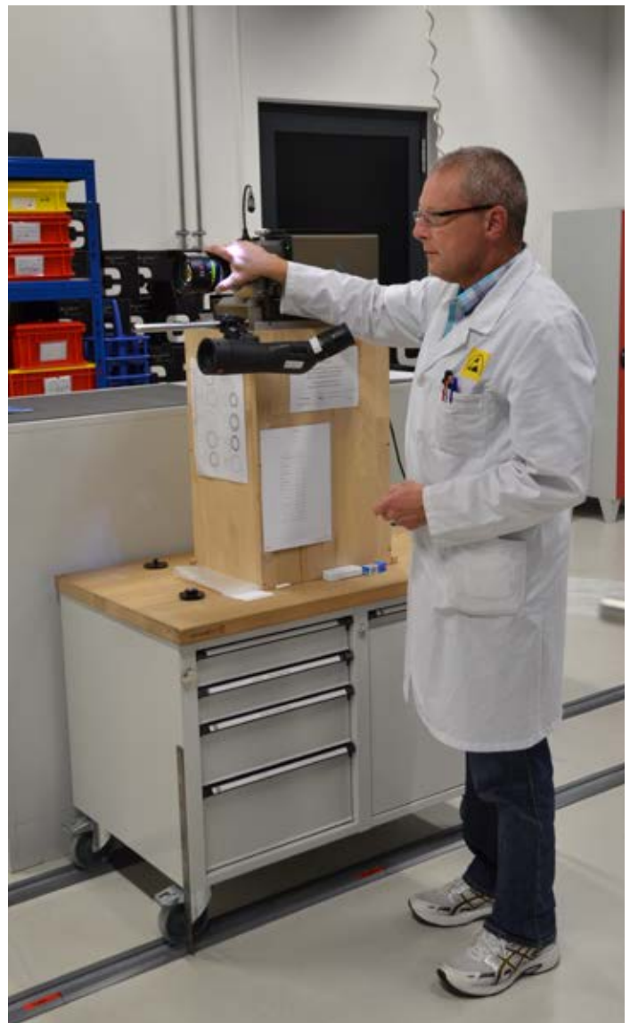
Lenses are checked on the lens projector at several intervals during the assembly process.
