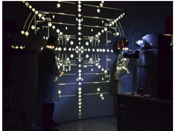
After mechanical wear-and-tear marathons, lenses are projected again.
