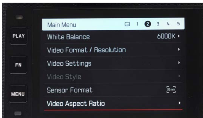
16. VIDEO ASPECT RATIO: push joystick to select one or more framelines. This does not crop or window the recorded image.
