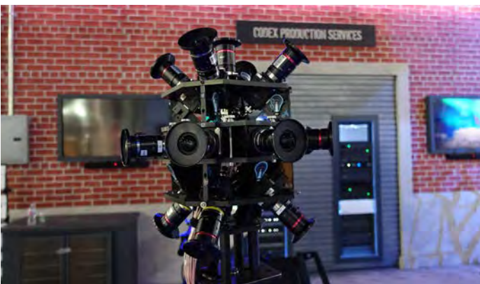
Codex- Radiant Images VR rig with 17 Codex Action Cameras: 360 degrees, 12-bit RAW files, C-mount lens. Jens Rumberg, Codex, at right.
