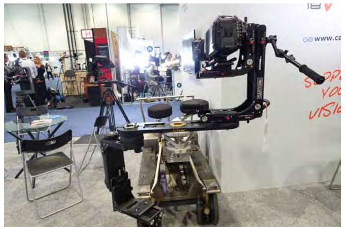
Lambda 25 Head is for cameras up to 25 kg (55 lb)
