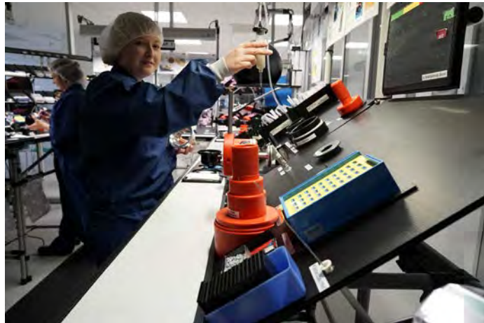
Barrel assembly of ZEISS Compact Prime lenses.
