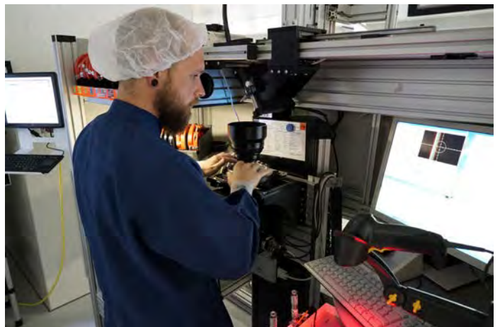
Checking the optical centering and finishing a Compact Prime.
