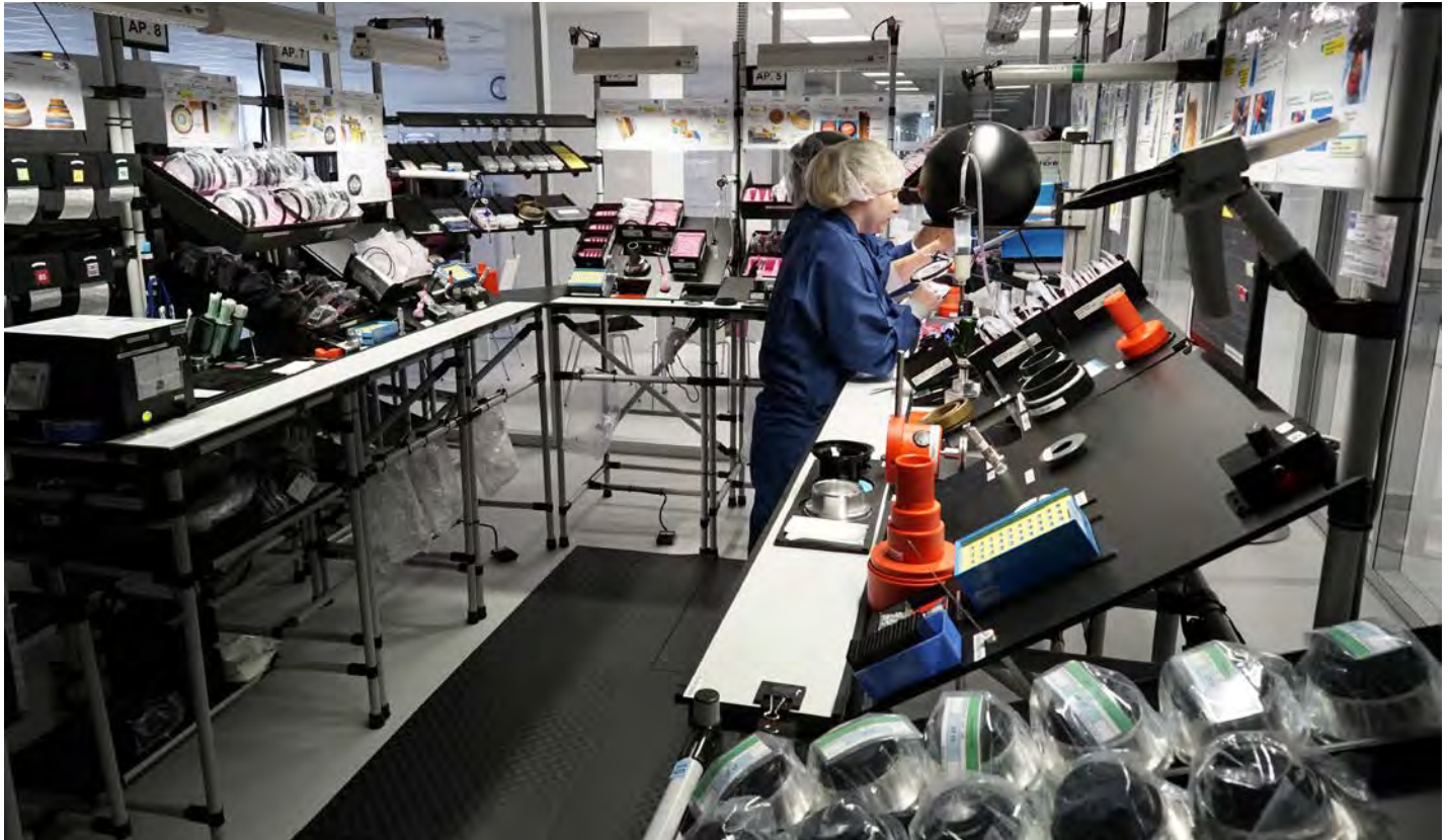
One piece flow: U-shaped work area. All parts and tools are within 25 cm reach. That's the reason the work surface is angled.
