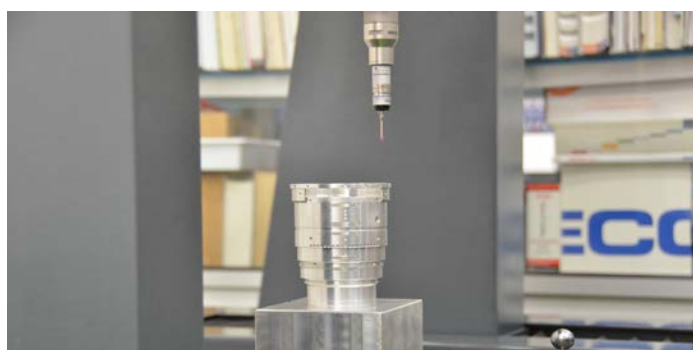
13. Measuring to 5 micron tolerances.
