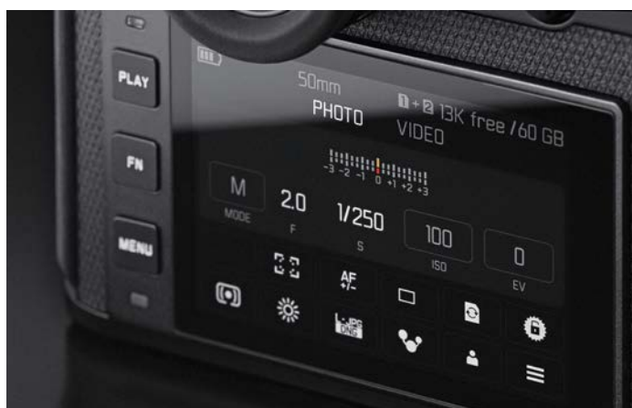
Photo Mode, above, showing 1/250 sec shutter speed, 100 ISO, etc. Video Mode, below: 180° shutter, 400 EI / ASA, timecode, audio levels.
