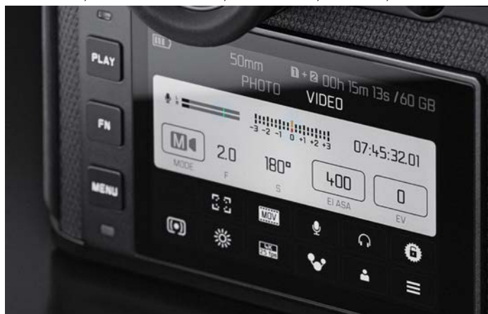
Photo Mode, above, showing 1/250 sec shutter speed, 100 ISO, etc. Video Mode, below: 180° shutter, 400 EI / ASA, timecode, audio levels.
