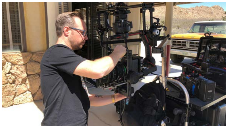
Above: Operator Andy DePung balances his DJI Ronin rig with a “stand-In” Premista pre-prototype 80-250mm on a Sony VENICE Rialto setup. Both Premistas are the same length and weight. The lens “stand-in” allowed production to move faster by having the next camera setup balanced and ready to go. Below: Aisha Schliessler viewing monitor.
