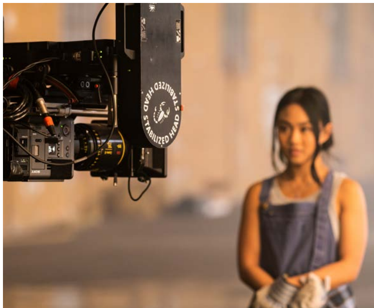
Scorpio Head underslung and camera upside down to get low to ground.
