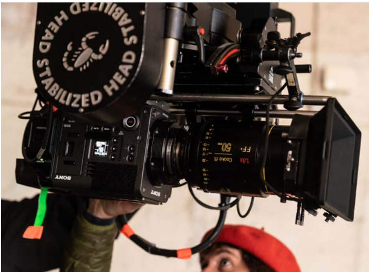
Scorpio Stabilized Remote Head underslung; VENICE and Cooke inverted.
