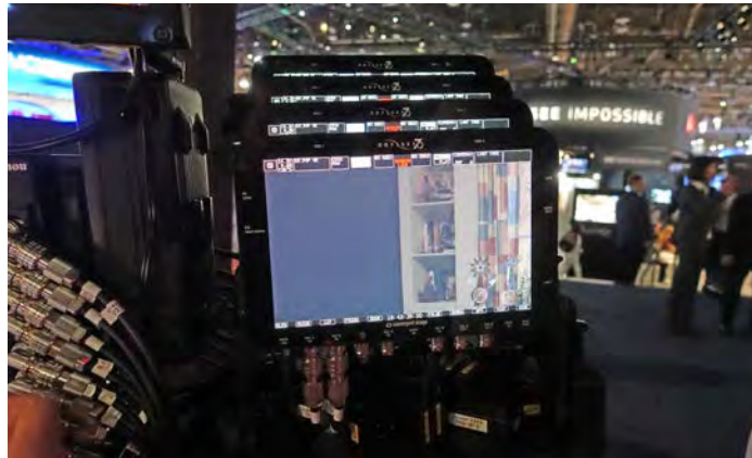
Four Convergent Design Odyssey 7Q Recorders are connected for 8K RAW capture. A 35.4 Megapixel still image can be saved from RAW.
