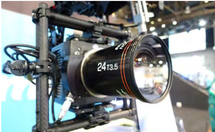
Prototype Panavision 24mm T3.5 lens on an ARRI Alexa Mini on a Gryphon Dynamics Drone. It appears to be weather-protected, aerodynamic, and without moving parts or barrels on the outside.
