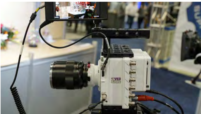
Vision Research Phantom VEO 640S has a 35mm 2.5K sensor, on-camera controls, CFast 2.0 media, weighs 5.6 lb (2.5kg) and is 5x5x5".
