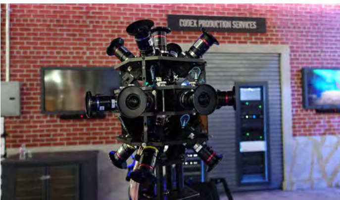
Codex- Radiant Images VR rig with 17 Codex Action Cameras: 360 degrees, 12-bit RAW files, C-mount lens. Jens Rumberg, Codex, at right.
