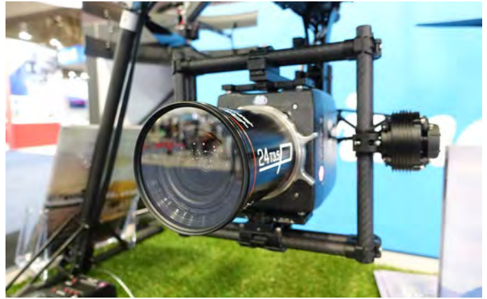
Prototype Panavision 24mm T3.5 lens on an ARRI Alexa Mini on a Gryphon Dynamics Drone. It appears to be weather-protected, aerodynamic, and without moving parts or barrels on the outside.
