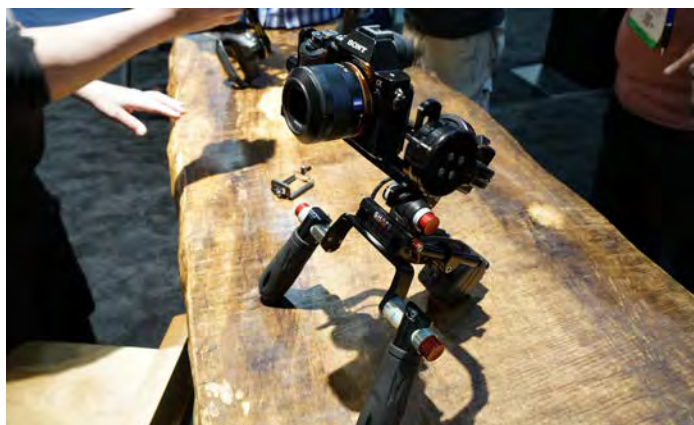
Shape Gimbal Handheld Small Body Camera Rig (2-axis: roll & tilt)
