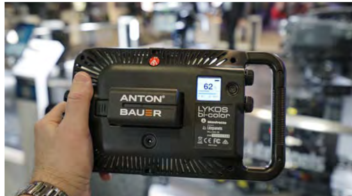
Litepanels Lykos Daylight and Bi-Color LED units draw 23 Watts, provide 1500 lux, measure 10.2 x 6 x 1.65" and weigh 1 lb
