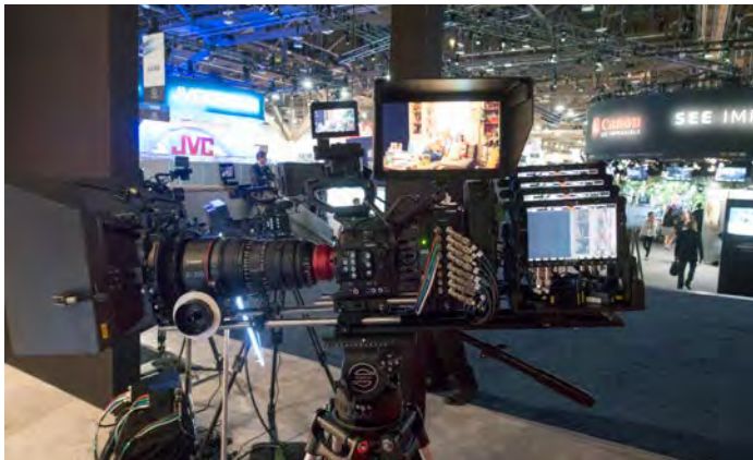
Working prototype 8K Canon camera, first shown at Canon Expo NY in September 2015. The 8K Super35 Sensor (8192 x 4329) outputs 8K RAW with a native ISO around 400 up to 60 fps.
