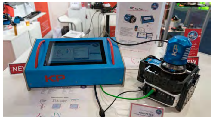
King Peter accurately measures the image sensor's position in digital cameras: center, rotation around the optical axis, and any deviation of the chip relative to a perpendicular image plane.
