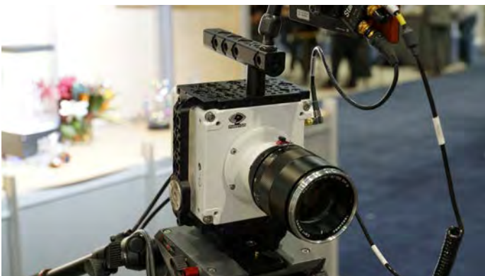
Phantom VEO 640 records up to 1400 fps at 2560 x 1600, 2500 fps at 1080p HD. With 72 GB of RAM at 1400 fps, record time is 8 secs.
