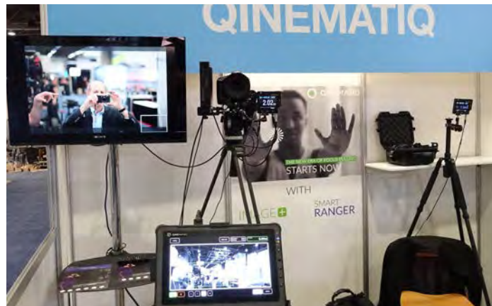
Martin Waitz and Verena Goetzner of Qinematiq, whose products are now distributed in the Americas by ZGC. Qinematiq's Image+ is a focus distance measuring device that uses its own real-time video image data to generate a 3D image map to determine focus of anything in the frame.
