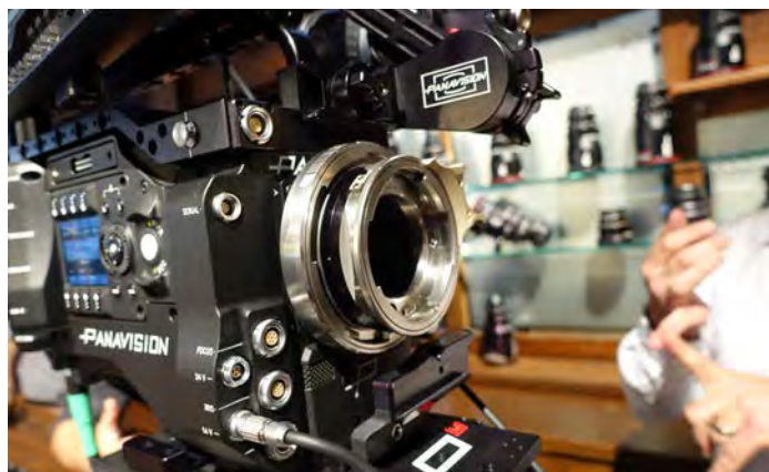
The DXL (40mm flange depth mount) with PV adapter
