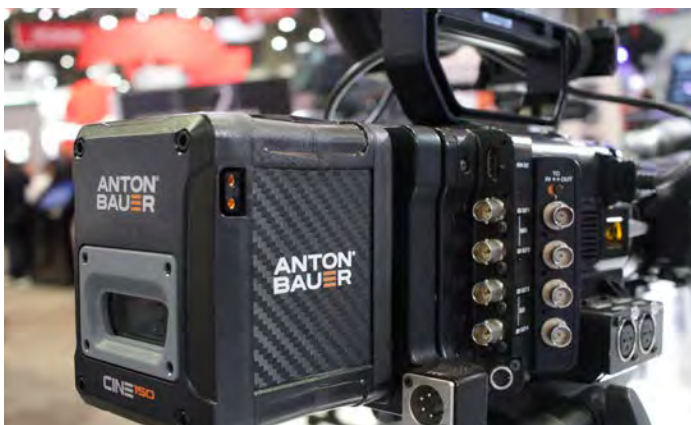
Anton Bauer Cine 150 14.4V 90Wh onboard battery
