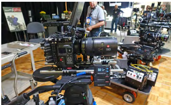
16x9inc Movcam accessories: wireless follow focus, handle, mattebox, power breakout box, with IB/E Optics Raptor FF Macro 180mm.
