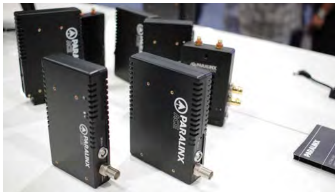
Paralinx ACE transmitters and receivers: up to 300 ft HD no latency
