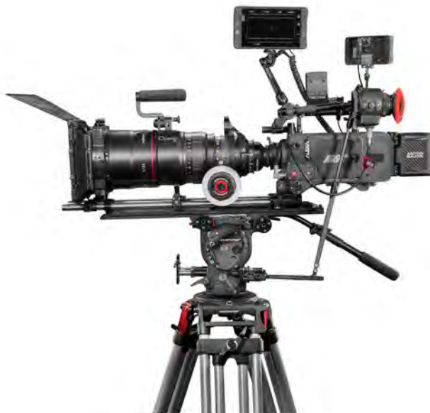
OConnor 2575D at 65% counterbalance, with ARRI Alexa, Angénieux 24-290 T2.8, OConnor CFF-1 Follow Focus, SmallHD monitors, Teradek, Anton Bauer onboard, Mattebox, Eyepiece leveler.
