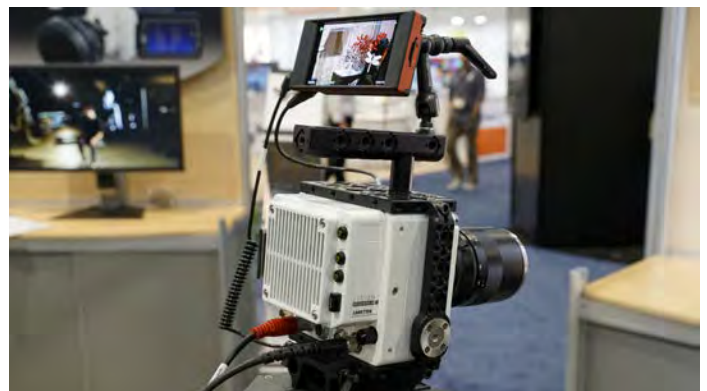
Vision Research Phantom VEO 640S has a 35mm 2.5K sensor, on-camera controls, CFast 2.0 media, weighs 5.6 lb (2.5kg) and is 5x5x5".
