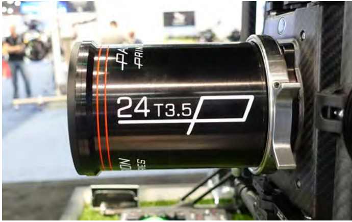
Prototype Panavision 24mm T3.5 lens on an ARRI Alexa Mini on a Gryphon Dynamics Drone. It appears to be weather-protected, aerodynamic, and without moving parts or barrels on the outside.
