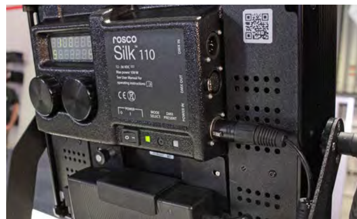
Rear of Rosco Silk 110, a 1x1 bicolor LED panel.
