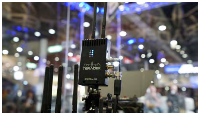
Teradek Bolt 600 Receiver. Transmitter range up to 600 ft.
