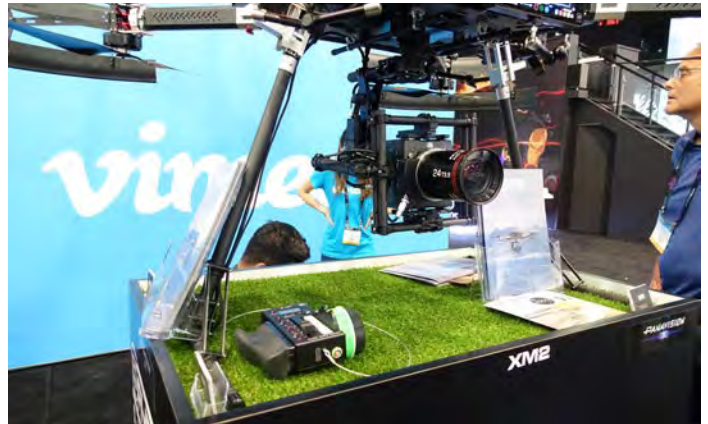
Prototype Panavision 24mm T3.5 lens on an ARRI Alexa Mini on a Gryphon Dynamics Drone. It appears to be weather-protected, aerodynamic, and without moving parts or barrels on the outside.
