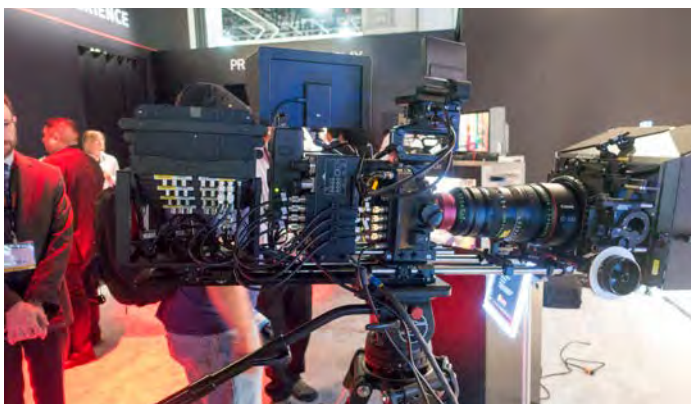
The lens shown here is a CN-E 30-300mm T2.95-3.7 L S EF Mount Cinema Zoom Lens. Note the locking ring on the ruggedized EF Mount.
