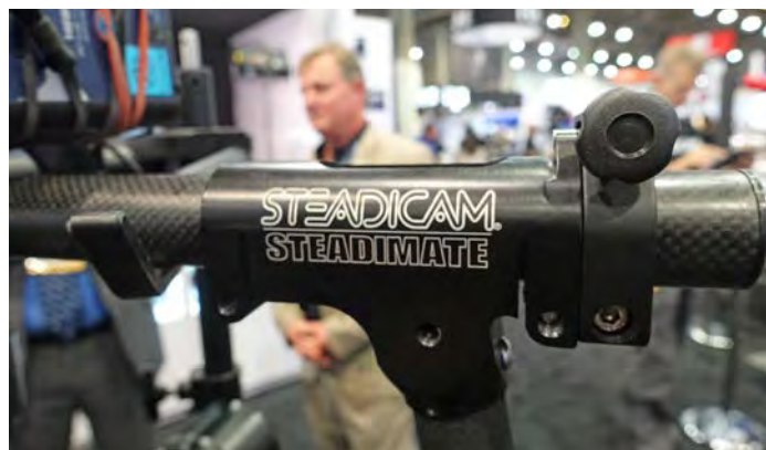
Tiffen Steadicam Steadimate mates motorized gimbals to the Steadicam
