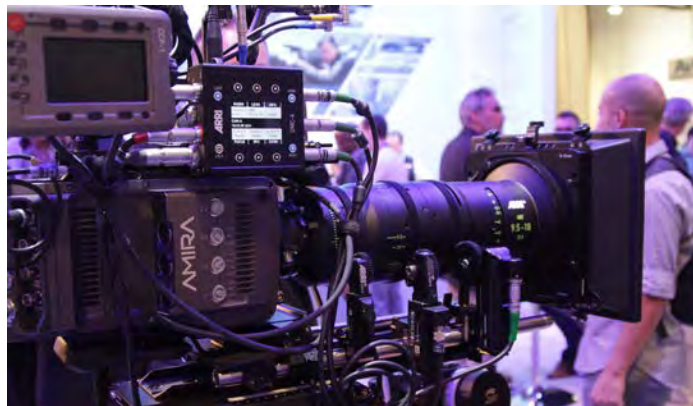
ARRI CCP-1 does the job of the MVF-1 — a 3.2" display for viewing and menu, but without the eyepiece. A popular accessory for Alexa Mini and Amira. The Universal Motor Controller UMC-4 is a wireless receiver for remote focus, iris and zoom control on any camera.
