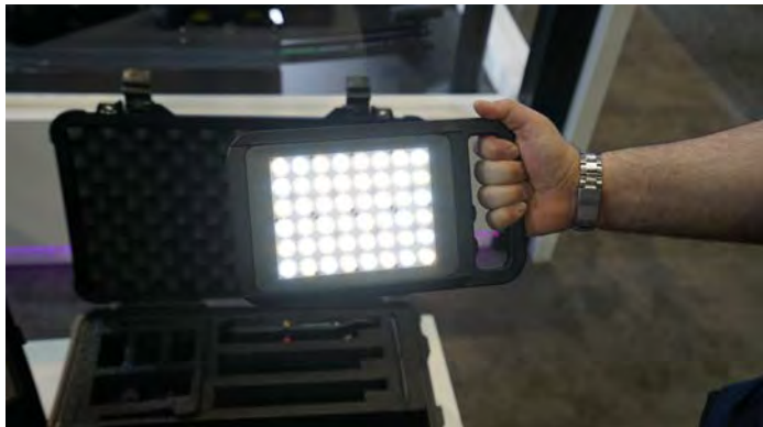
Litepanels Lykos Daylight and Bi-Color LED units draw 23 Watts, provide 1500 lux, measure 10.2 x 6 x 1.65" and weigh 1 lb
