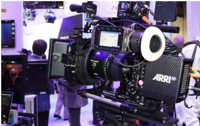
ARRI Alexa Mini with MVF-1 (Multi View Finder) is the same one that comes on Amira camera packages. The 3.2" LCD display swings out.
