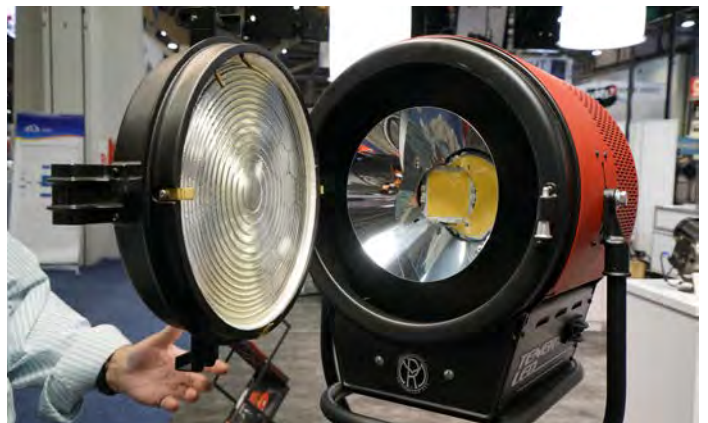
Light engine inside Mole Tener LED (equiv 10K tungsten)
