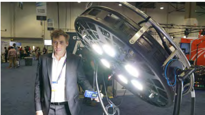
Tama Berkelson, MD of Outsight with Creamsource Sky: 1200W (equiv to 5K Tungsten) adjustable 2,200-15,000K and adjustable Green/Magenta.
