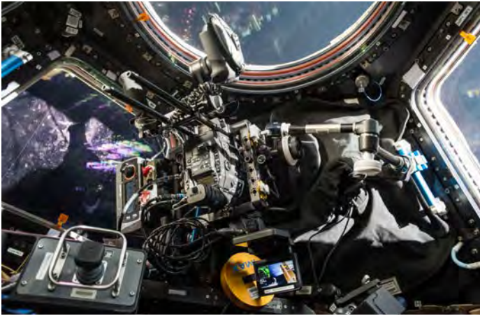
The C500 is secured to the wall with Magic Arms (formerly from Bogen, now Manfrotto). One end attaches to the 1/4-20 thread on the camera and the other end fits into the "seat track" – a running set of rails to which the arms can be mounted anywhere in the ISS. Photo: NASA
