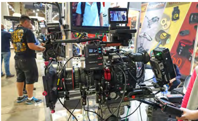
16x9inc Movcam accessories: wireless follow focus, handle, mattebox, power breakout box, with IB/E Optics Raptor FF Macro 180mm.
