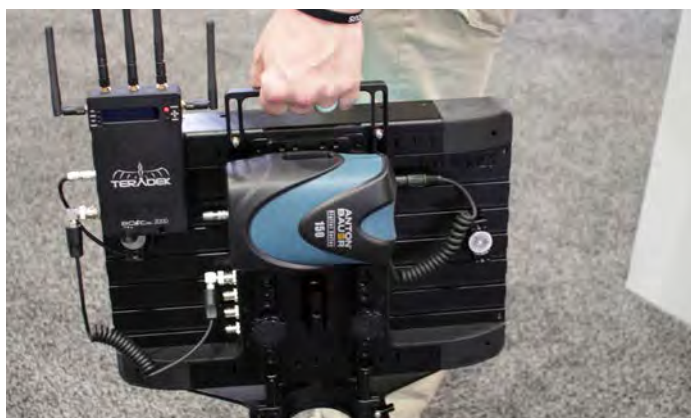
SmallHD Production Monitors have rugged aluminum chassis, carrying handle, stand, and mounting rails for wireless receivers, batteries, etc.
