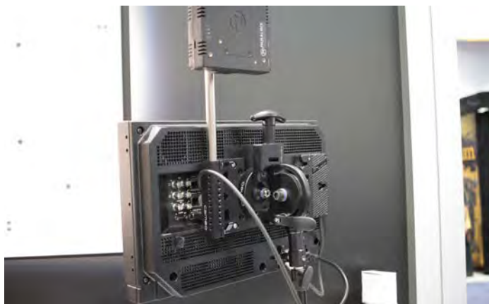
AbelCine Cameo VESA Mount for monitors up to 25"
