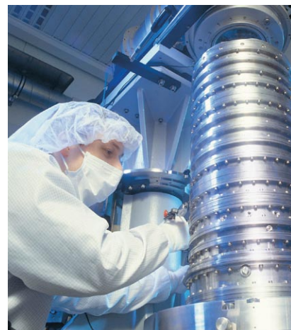
Carl Zeiss Semiconductor lens. 870 kg.
