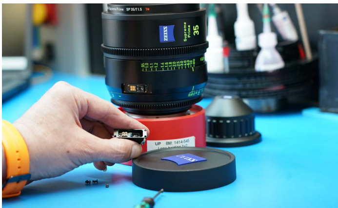
Connector removed, revealing electronics board beneath.
