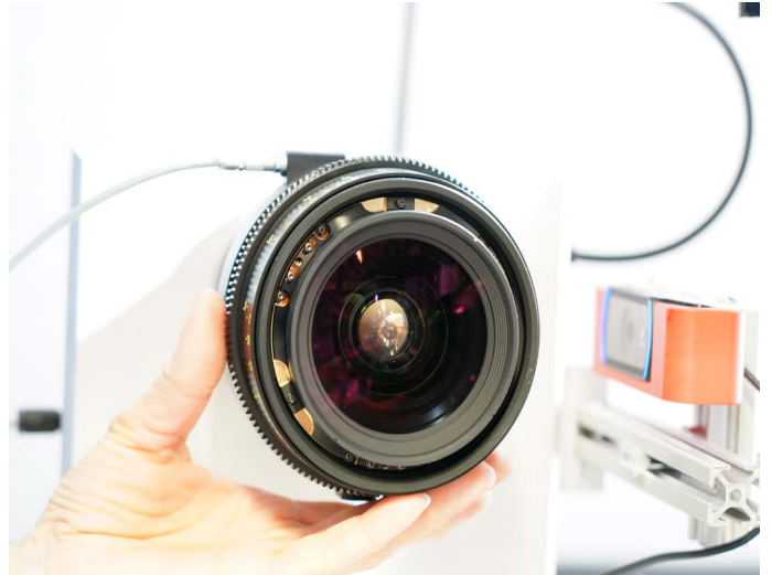
Focus and iris marked are checked against the XD metadata
