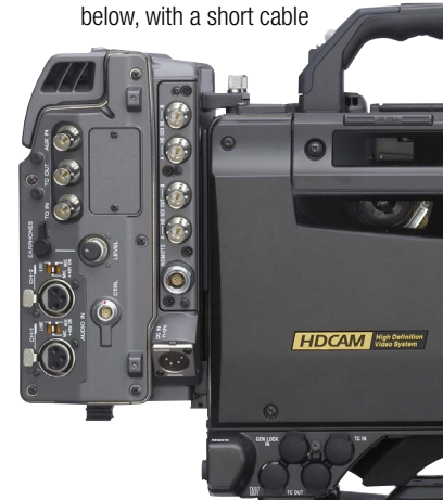
SR-R1 connects to F900, below, with a short cable
