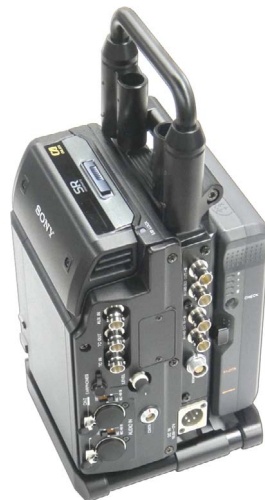
SR-R1 Memory Recorder at left, with brackets to mount on camera support rods of cameras like the F3, connects via SDI.
