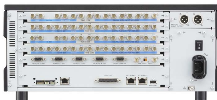
SR-R1000 Multi-Card Ingest / Multi Channel Server stores 12TB, about 12 hours of 4K content.
