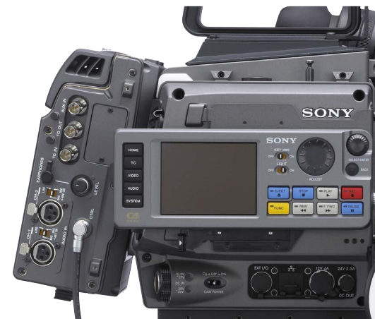
SR-R3 Memory Recorder directly connected to F35, above and below.
