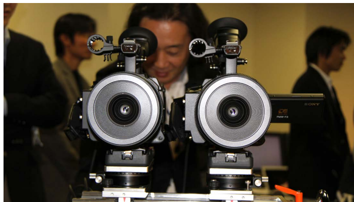
Above: Two F3 cameras set up on a 3D side-by-side rig.
