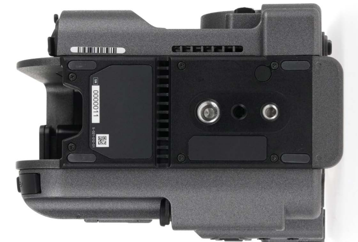
Bottom View showing Mounting Threads. Front of Camera is at Right.
