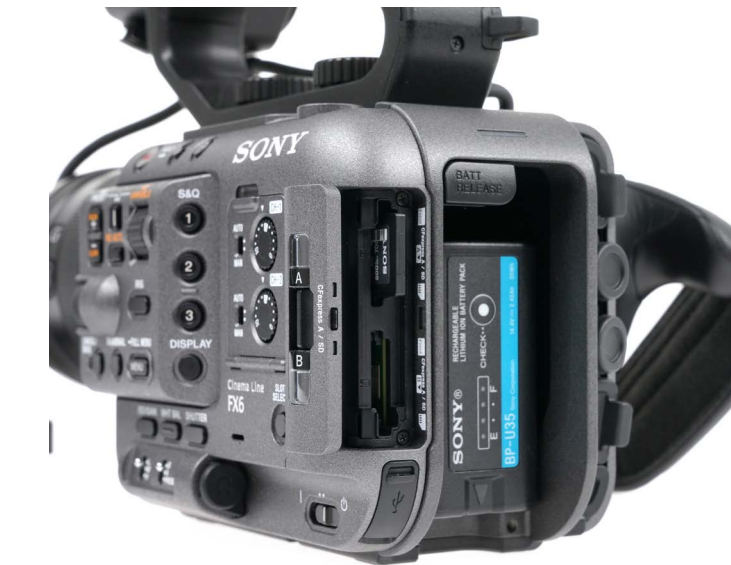
Detail of CFexpress and SD Slots with Door Open and Battery in Place.
