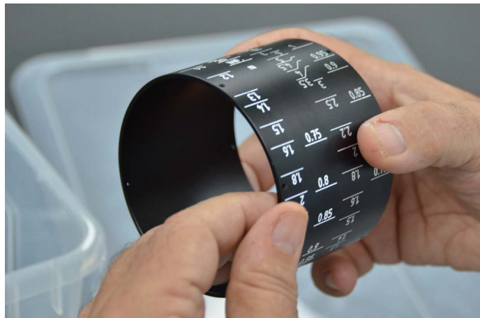
3. The barrel goes downstairs for engraving, then returns to the lens assembly room upstairs.
