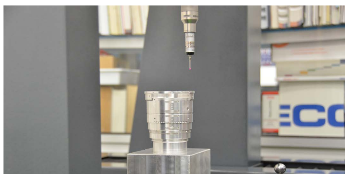
13. Measuring to 5 micron tolerances.
