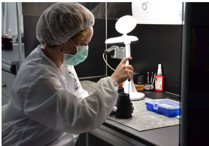
Above: Mounting optical assemblies in lens barrel. Below: QC and measuring optical elements.
