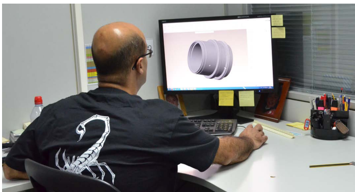
5. Above: because Scorpio remote heads require CNC machining to less than 5 micron tolerance, work on lens barrels is business as usual, and done entirely in house. 6. Below: design is transferred to CNC machine.
