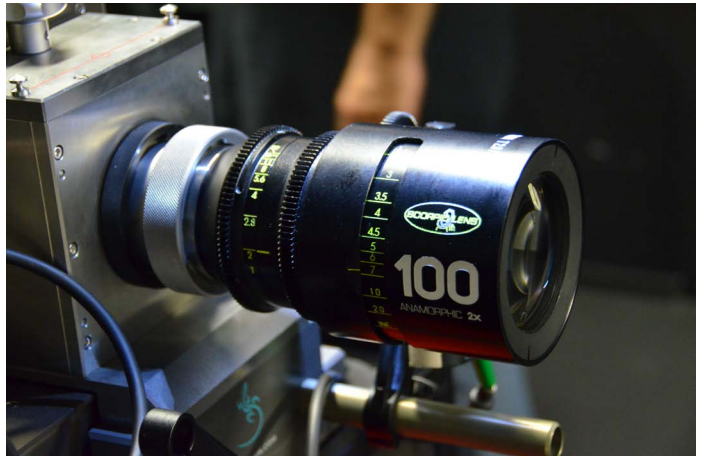
4. The engraved barrel is installed and tested again.
