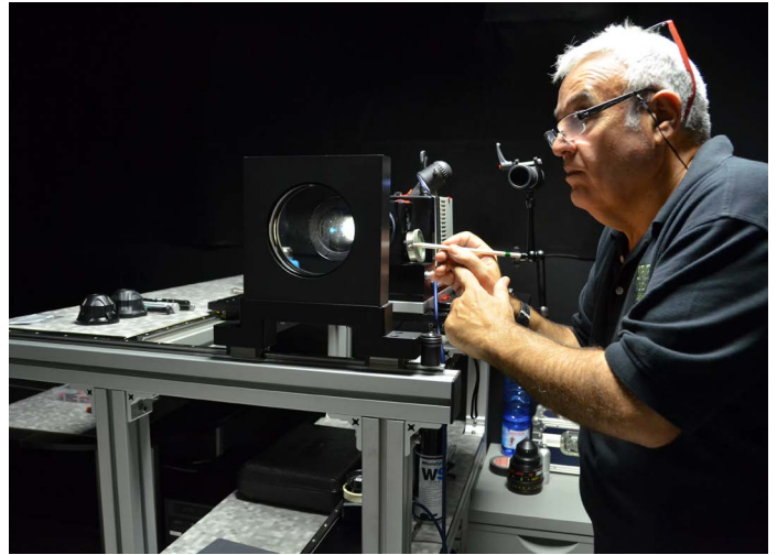
2. Each mark is scribed with a white marker. A moveable diopter slides in front of the lens for far distance marks.
