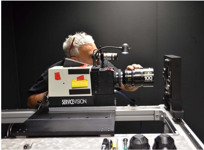
1. In a room adjacent to the clean room, Andres projects each lens to calibrate the focus scale. He uses a monocular for viewing.
