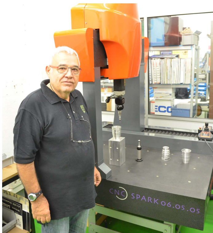
11. Above: Andres Valles measuring accuracy of machined barrels.
