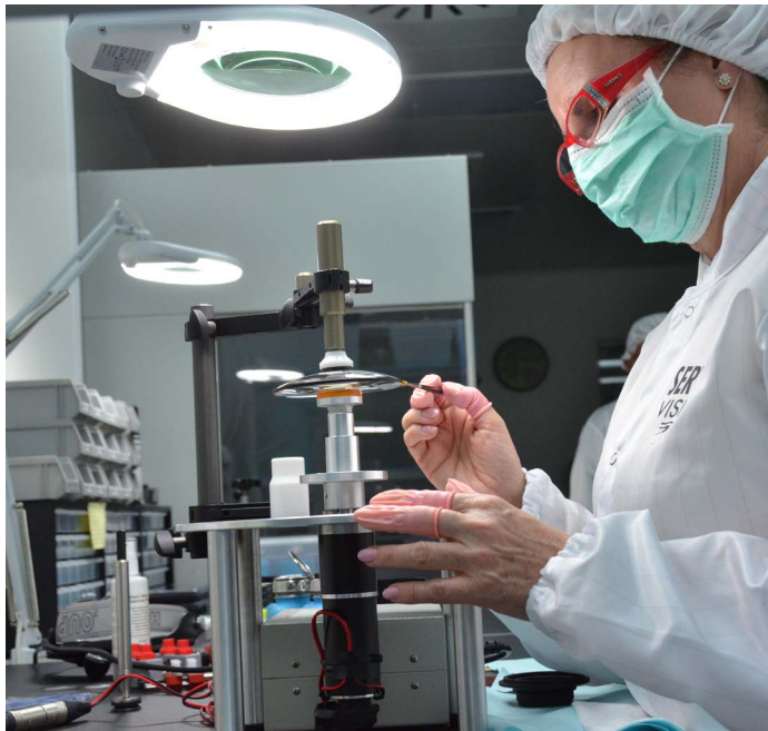
Above: Blacking edges of optical elements.
