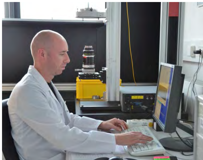
Measuring air gaps of completed lens
