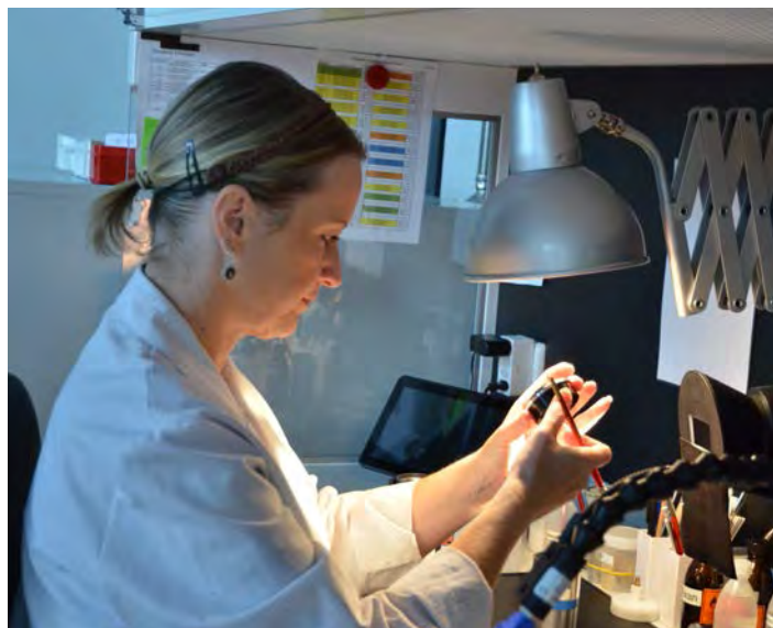
Cleaning and inspecting optical elements
