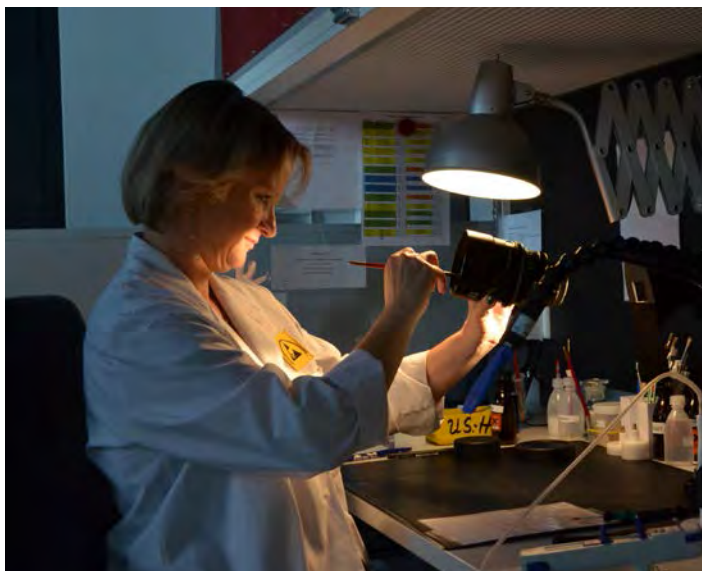
Cleaning optical sub-assemblies
