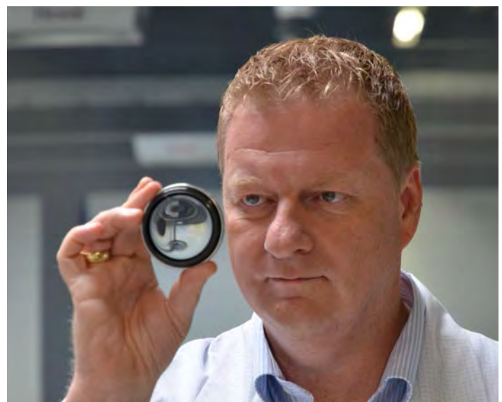
Bernhard Kratzer inspecting an aspherical element. You can tell it’s an asphere by the concentric rings.
