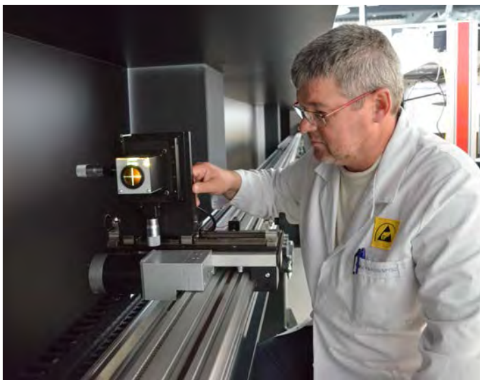
The target is controlled from the computer, moving to the pre-determined distance for each focus mark calibration.
