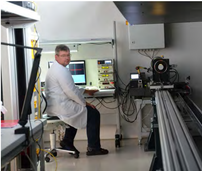
A focus-scale indexing system on a 60' long "railroad" moves an MTF target to each marked distance to be engraved on the focus barrel.
