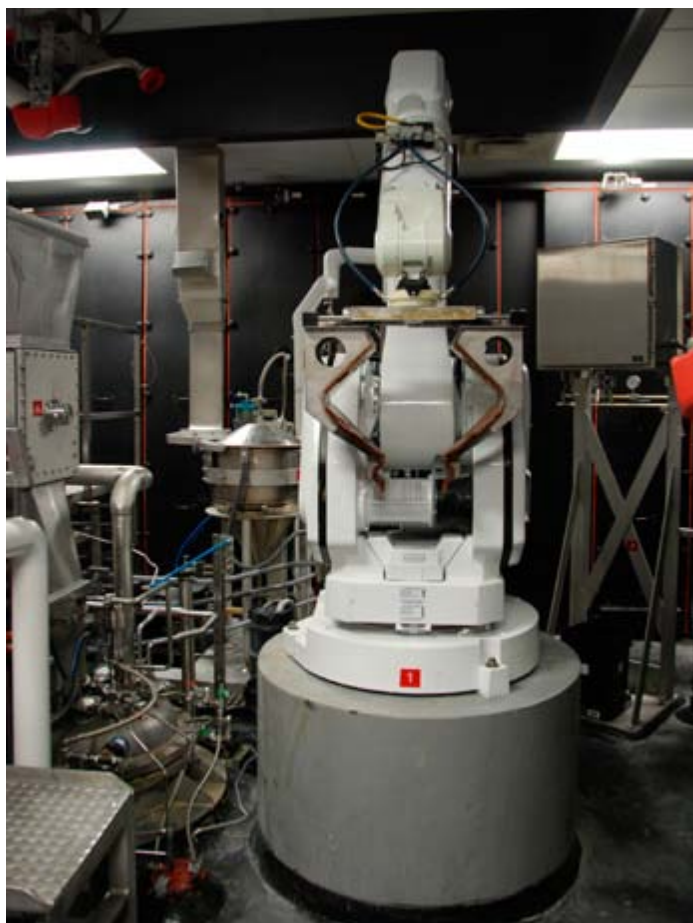
Robots eliminate variability: handling, mixing, and pouring the ingredients for the layer parts.
