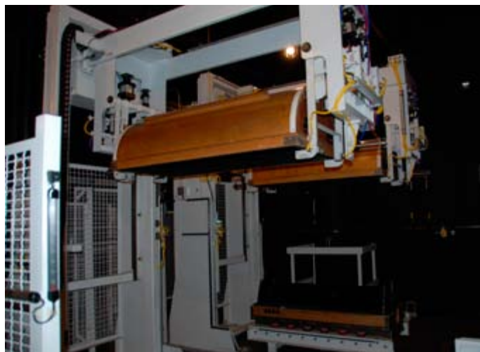
The 6,000' master rolls are removed from the containers (in the dark) and prepared for slitting.
