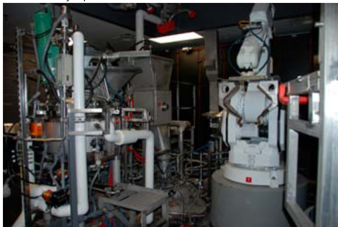
Robots eliminate variability: handling, mixing, and pouring the ingredients for the layer parts.
