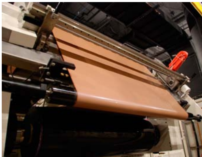
The 6,000' master rolls are removed from the containers (in the dark) and prepared for slitting.
