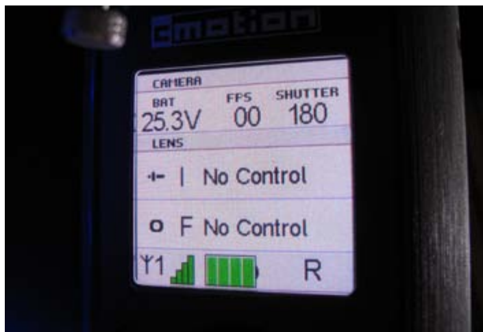
The evolution main display, showing camera power, fps, shutter, wireless signal strength, evolution battery status, lens information and more.
