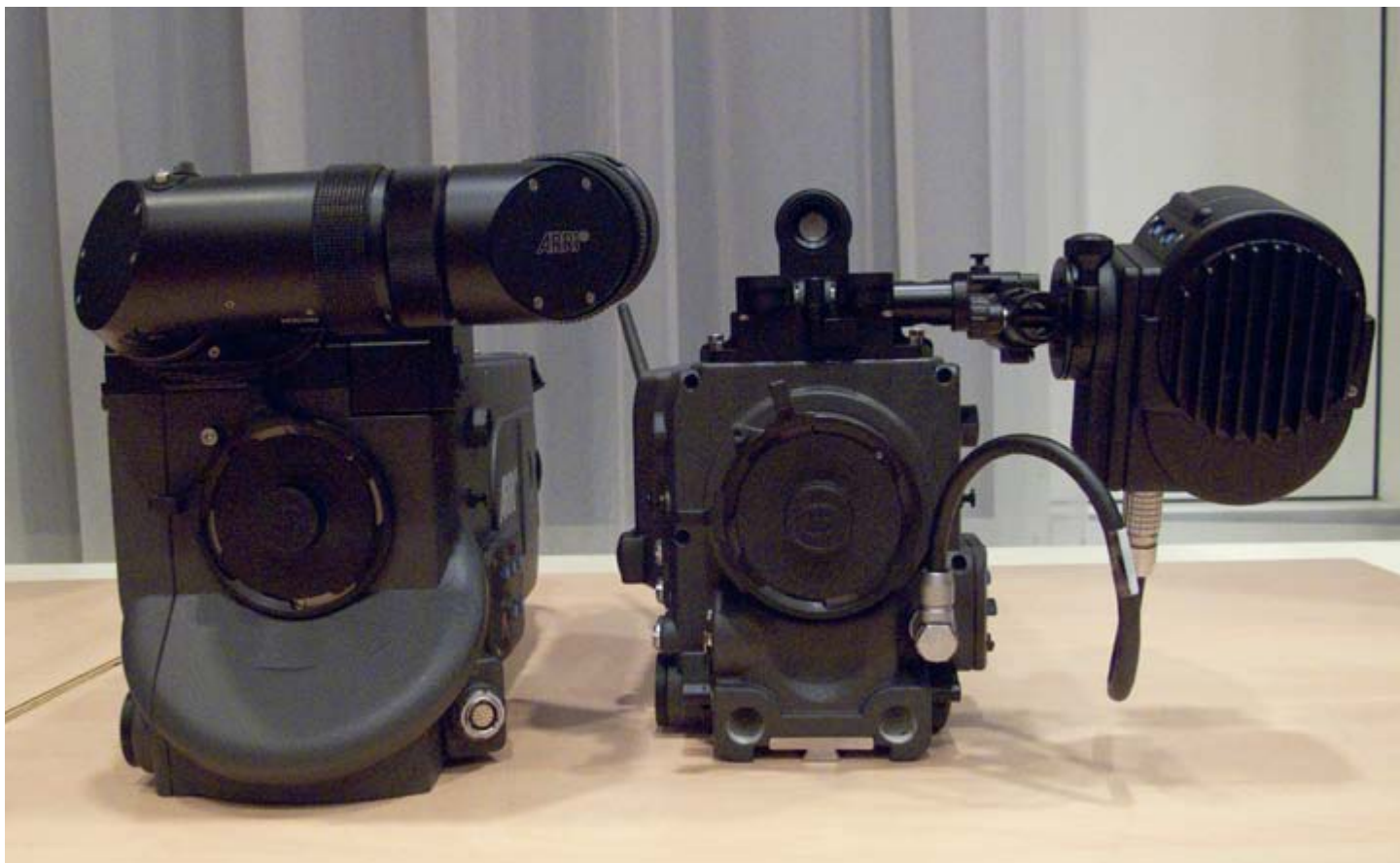
Above: front view of Alexa EV pre-prototype with electronic finder, and lightweight 15mm supports under PL mount.
